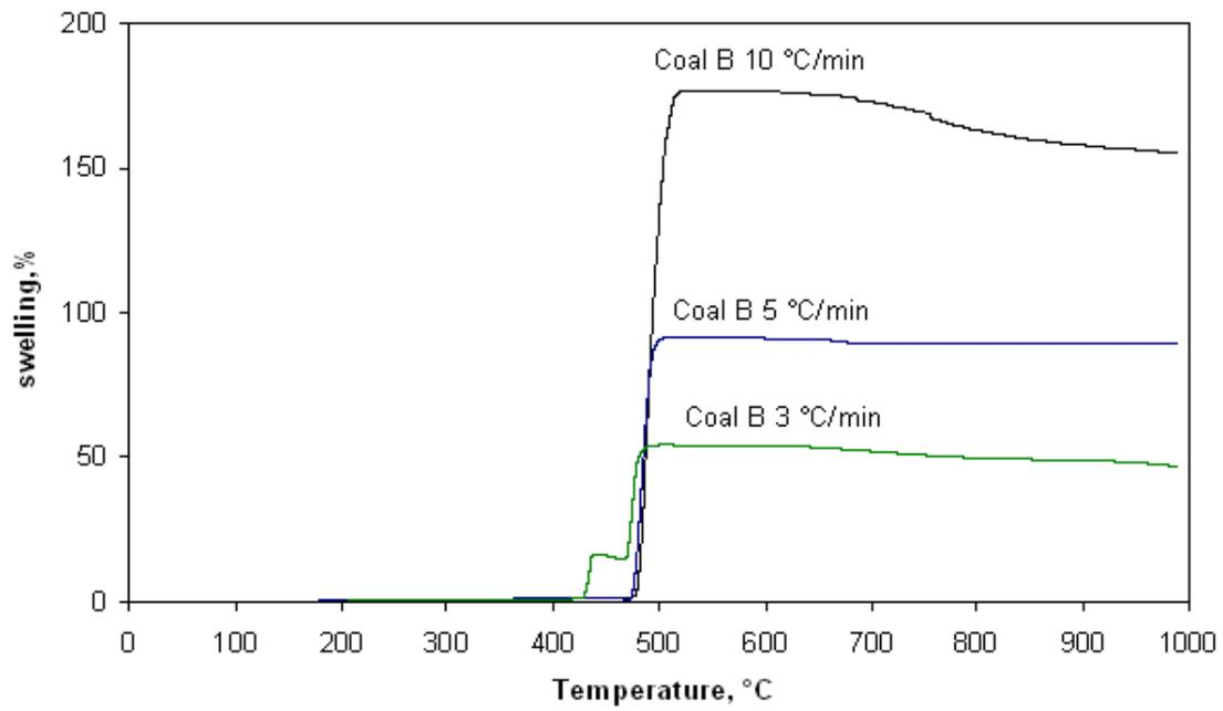
Figure 4.8. Swelling of coal sample B at three different heating rates of 3, 5 and 10°C/min from 25 to 1000°C.
