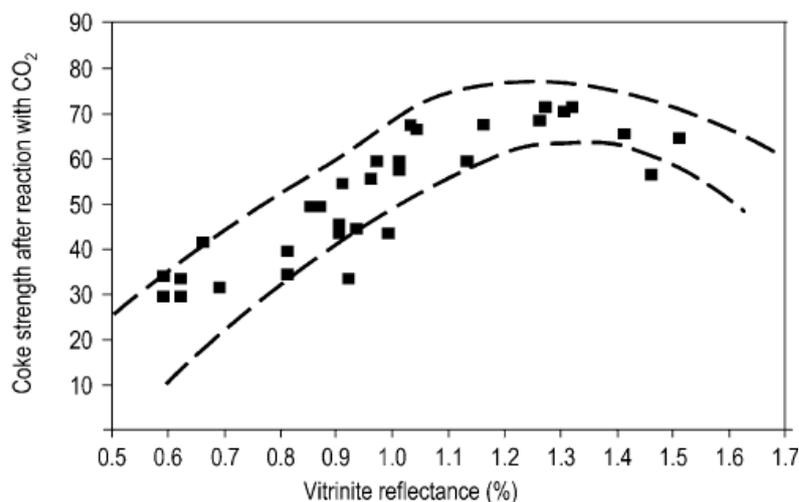
**Figure 2.13. Relationship between vitrinite reflectance and coke strength after reaction with carbon dioxide (CSR) [7].**
