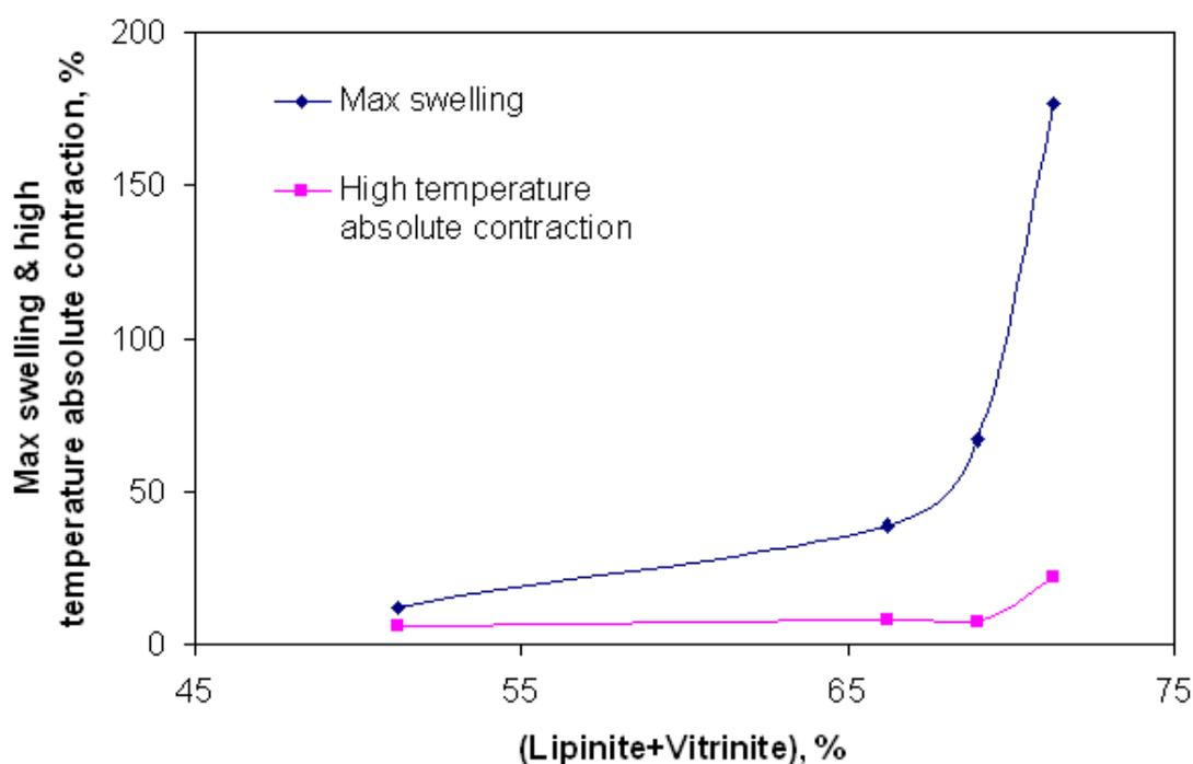
**Figure 4.2. Relationship between maximum swelling and high temperature absolute contraction with vitrinite plus liptinite content for four coal samples at a heating rate of 10°C/min from 25 to 1000°C.**
