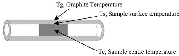
Figure B.4. Schematic representation of measured temperatures for heating sample.
