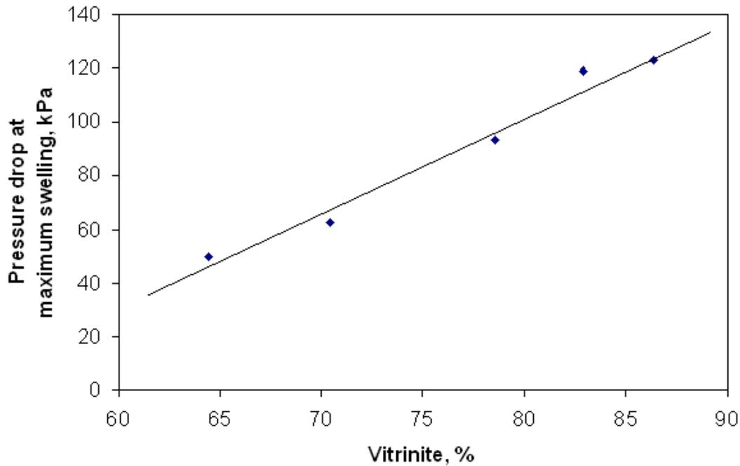
**Figure 7.10. Relationship between pressure drop of gas flowing through the coal sample at maximum swelling and vitrinite content for coal maceral concentrates at a heating rate of 10°C/min.**
