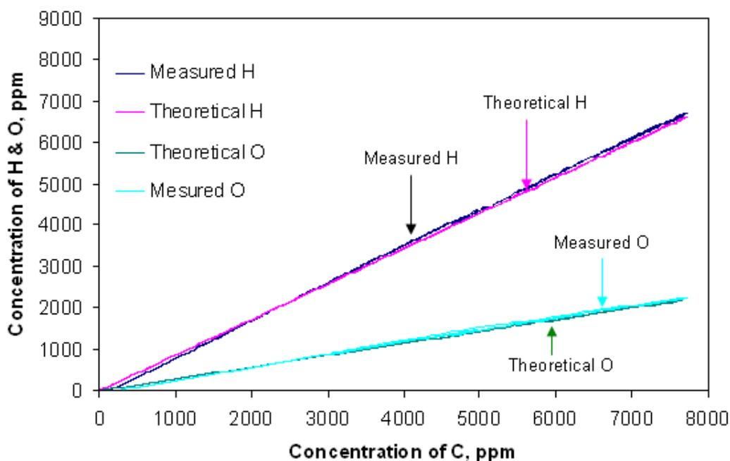
Figure A.6. Elemental evolutions for benzoic acid combustion at a heating rate of  $10^{\circ}C/min$ .
