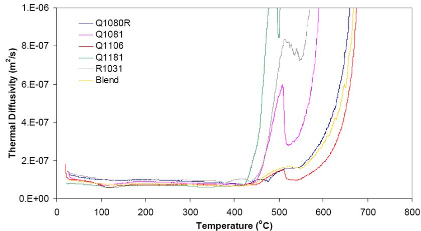
**Figure 2.17. Effective thermal diffusivity for the coal samples at a heating rate of 5°C/min heated from room temperature to 1000°C [19].**
