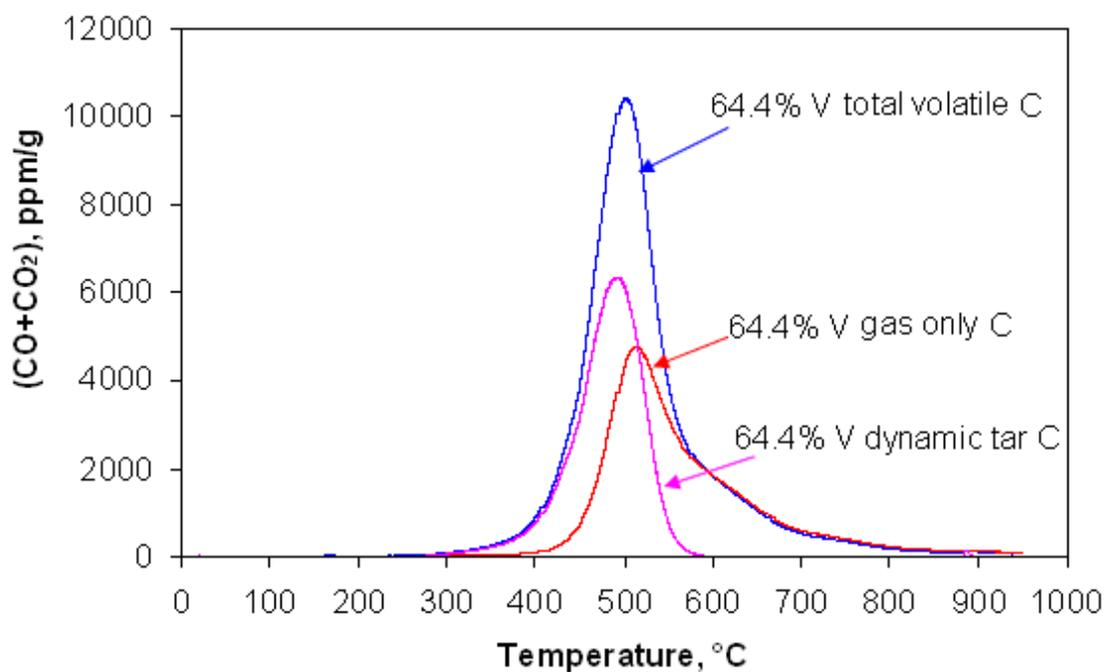
Figure 8.8. Carbon concentration for total volatile, gas only and mathematically derived dynamic tar for the 64.4% vitrinite concentrate at a heating rate of 10°C/min from 25 to 1000°C.
