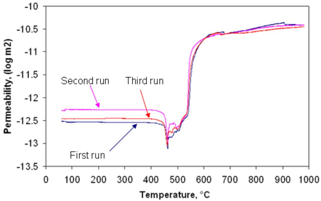
Figure 7.3. Permeability of the 86.4% vitrinite concentrate at a heating rate of 10°C/min from 25 to 1000°C for three replicate experiments.
