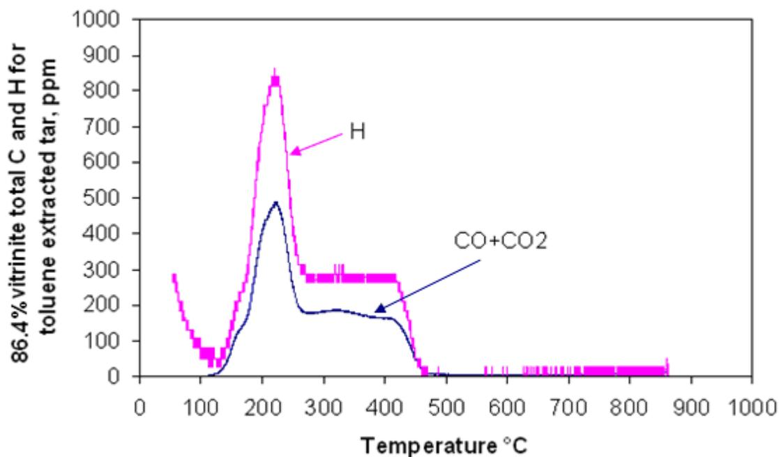
Figure 8.27. Properties of toluene extracted tar obtained from the 86.4% vitrinite concentrate at a heating rate of 10°C/min from 25 to 505°C.
