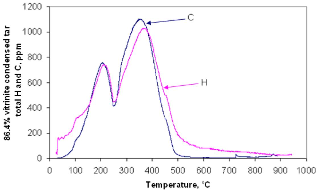
Figure 8.20. Properties of condensed tar obtained from the 86.4% vitrinite concentrate at a heating rate of 10°C/min from 25 to 1000°C.
