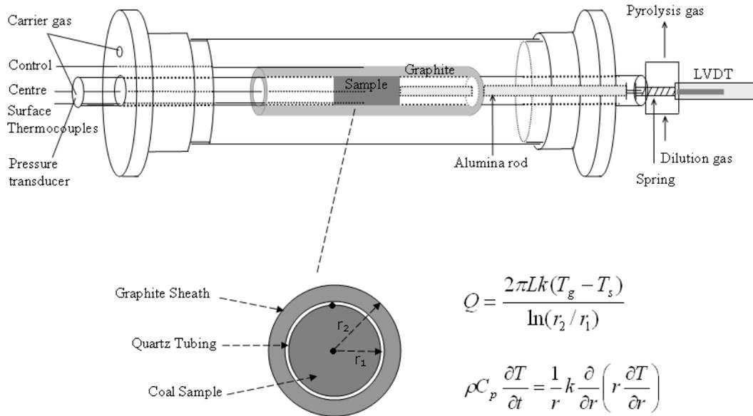
**Figure 3.2. Schematic representation of the thermo-swelling test setup.**
