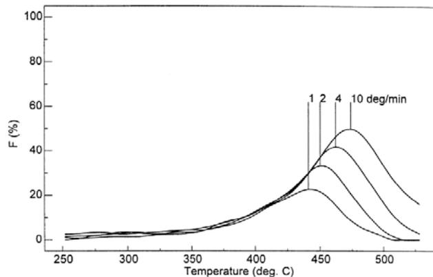
**Figure 2.5. Effect of heating rate on fusibility of a coal (74% vitrinite) [91].**
