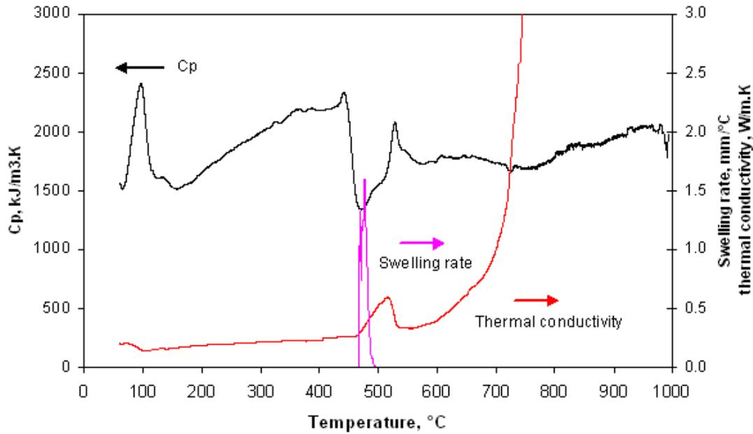
**Figure 4.7. Correlations between the apparent specific heat, thermal conductivity and swelling rate with temperature for the coal sample E at a heating rate of 10°C/min from 25 to 1000°C.**
