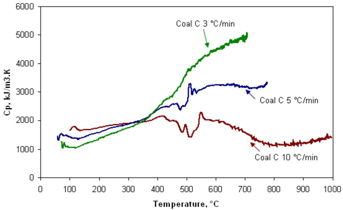
Figure 4.14. Apparent specific heat of coal sample C at three different heating rates of 3, 5 and 10°C/min from 25 to 1000 °C.
