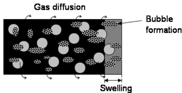
(c) Gas flow (mainly volatiles and some carrier gas) is restricted to diffusion through liquid metaplast and bubble formation (400-450°C) occurs, the swelling portion is indicated by a different colour to the original coal bed.
