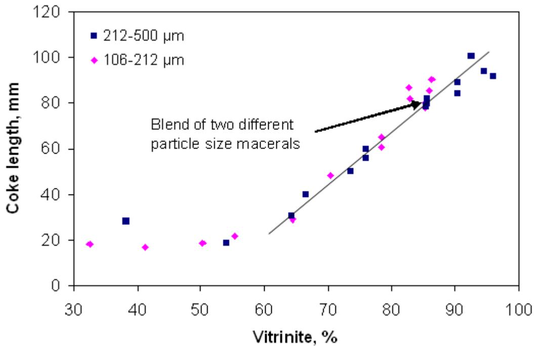
**Figure 6.22. Final coke length for all coal maceral concentrates at a heating rate of 10°C/min from 25 to 1000°C.**
