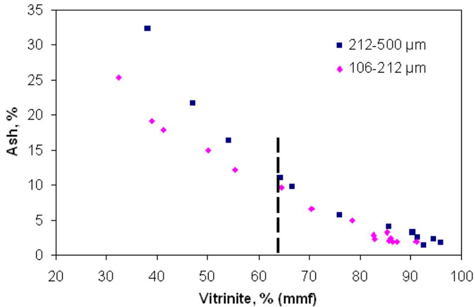
Figure 6.2. Relationship between vitrinite content and ash content for all 106-212  $\mu\text{m}$  and 212-500  $\mu\text{m}$  size cuts of coal maceral concentrates.
