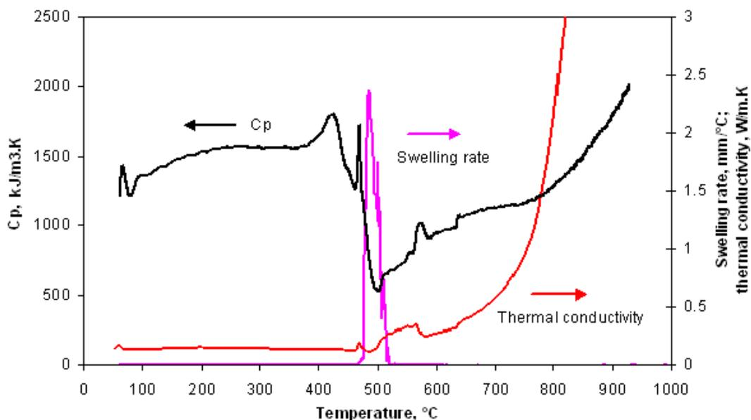
**Figure 4.6. Correlations between the apparent specific heat, thermal conductivity and swelling rate with temperature for coal sample B at a heating rate of 10°C/min from 25 to 1000°C.**
