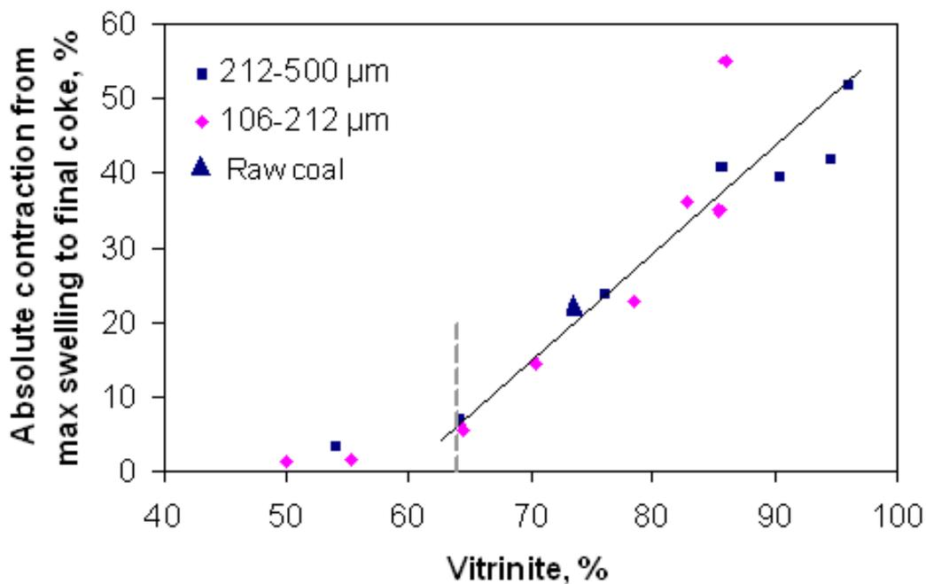
Figure 6.15. Relationship between vitrinite content and high temperature absolute contraction (550-1000°C) for the 106-212 μm and 212-500 μm size cuts of coal maceral concentrates at a heating rate of 10°C/min.
