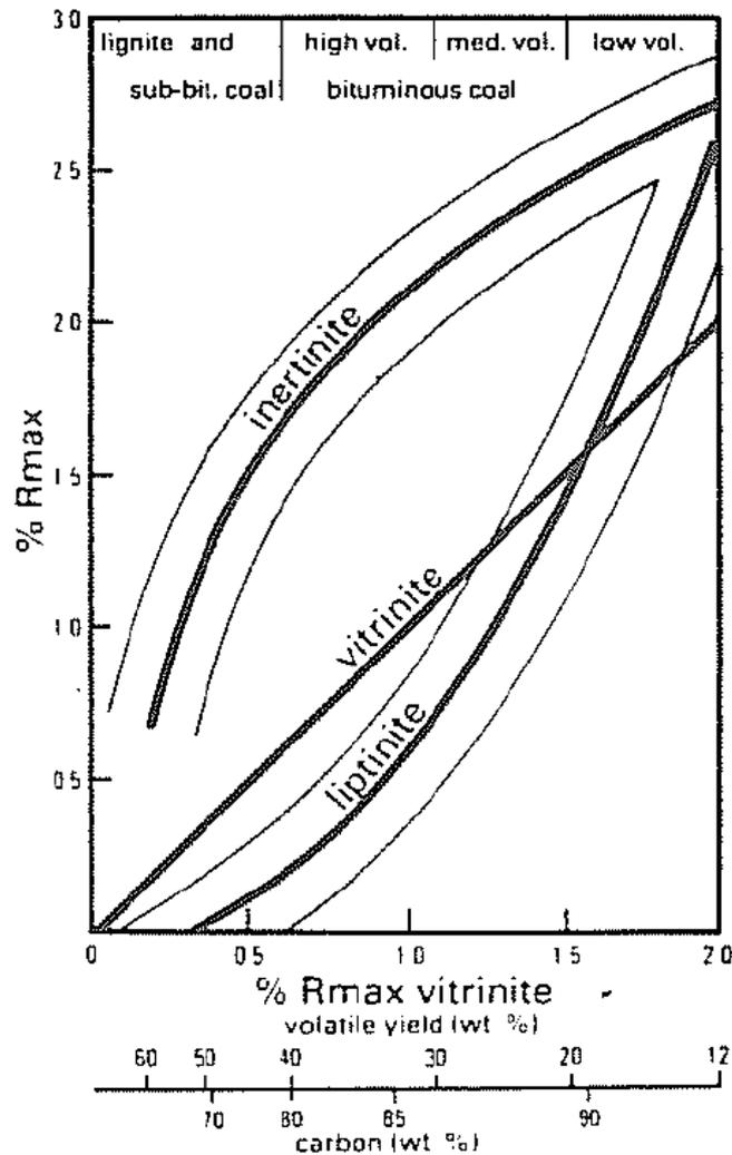
Figure 2.2. Reflectance of macerals as a function of coal rank, the maximum reflectance of vitrinite is chosen as a parameter for the coal rank,  $R_{Max}$  is mean maximum reflectance [27].
