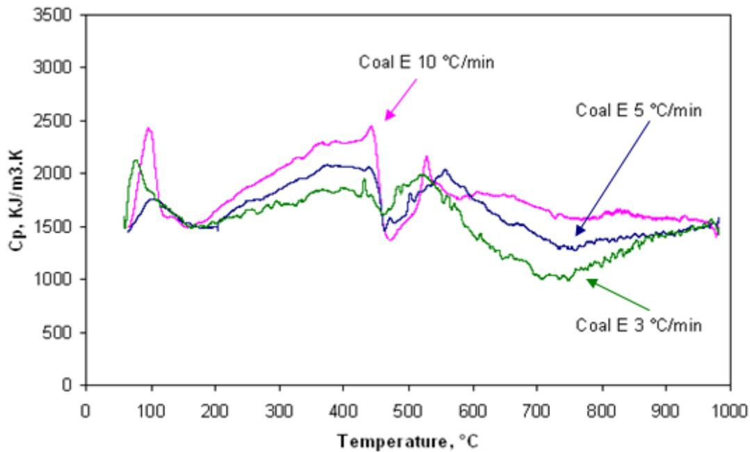
**Figure 4.16. Apparent specific heat of coal sample E at three different heating rates of 3, 5 and 10°C/min from 25 to 1000°C.**
