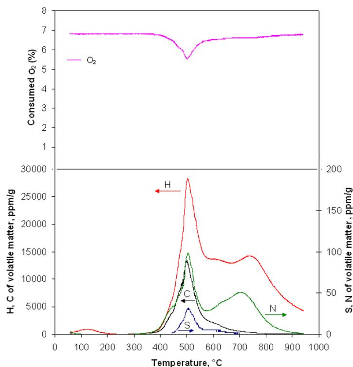
**Figure 8.1. Instantaneous elemental compositions of C, H, N, S and O by combusting volatiles released from heating the 86.4% vitrinite concentrate at a heating rate of  $10^\circ\text{C}/\text{min}$  from 25 to  $1000^\circ\text{C}$ .**
