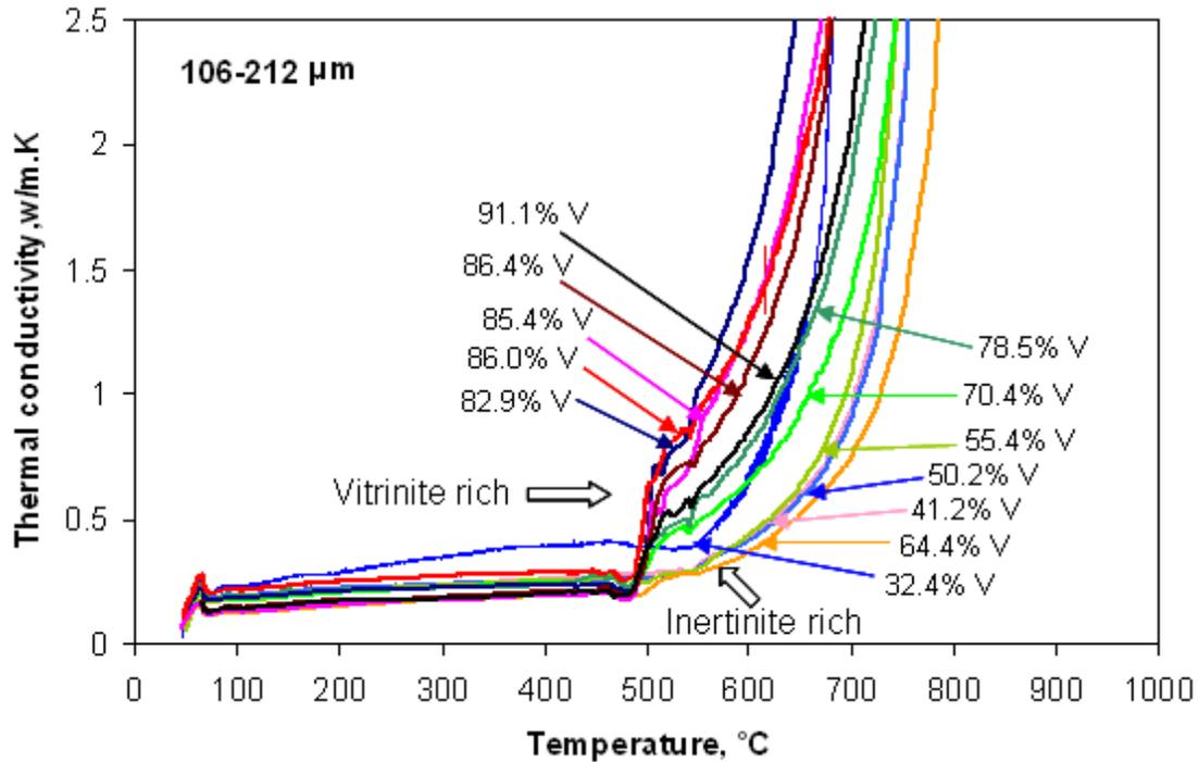
Figure 6.9. Thermal conductivity for 106-212  $\mu\text{m}$  coal maceral concentrates at a heating rate of  $10^\circ\text{C}/\text{min}$  from 25 to  $1000^\circ\text{C}$ .
