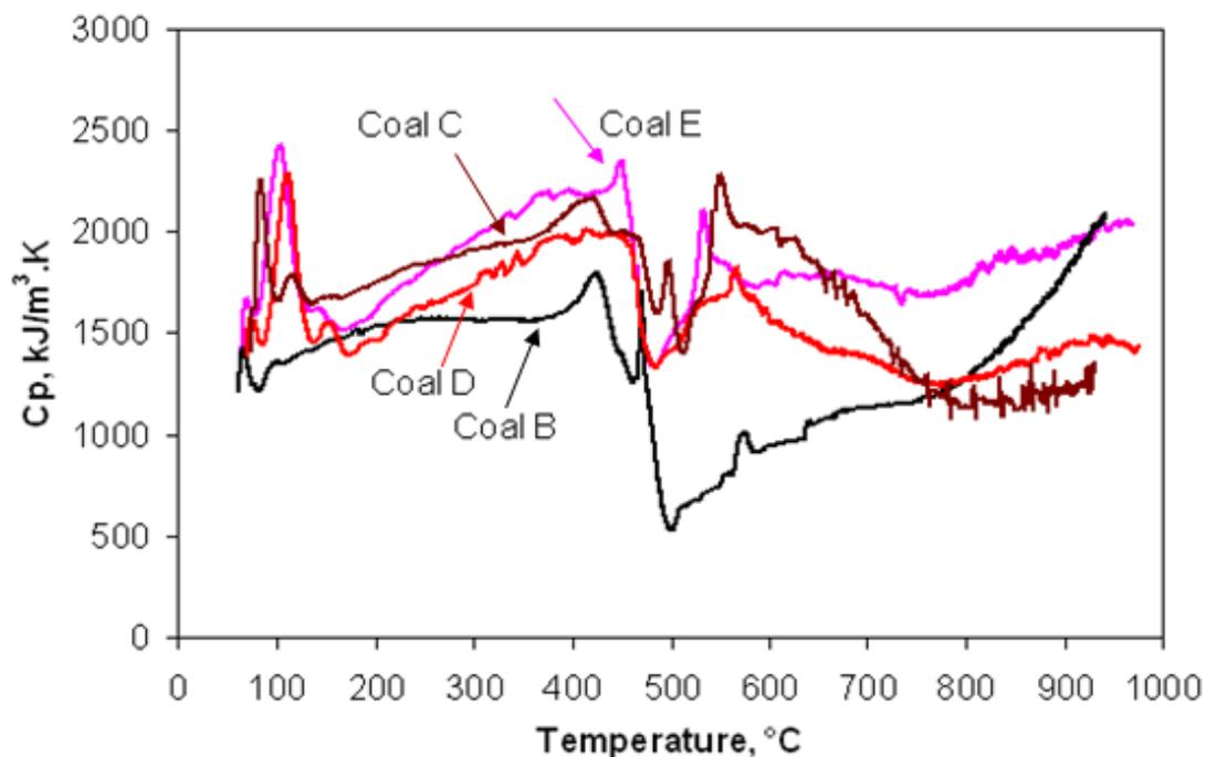
**Figure 4.3.** Comparison of the apparent specific heat for four coal samples at a heating of 10°C/min from 25 to 1000°C.
