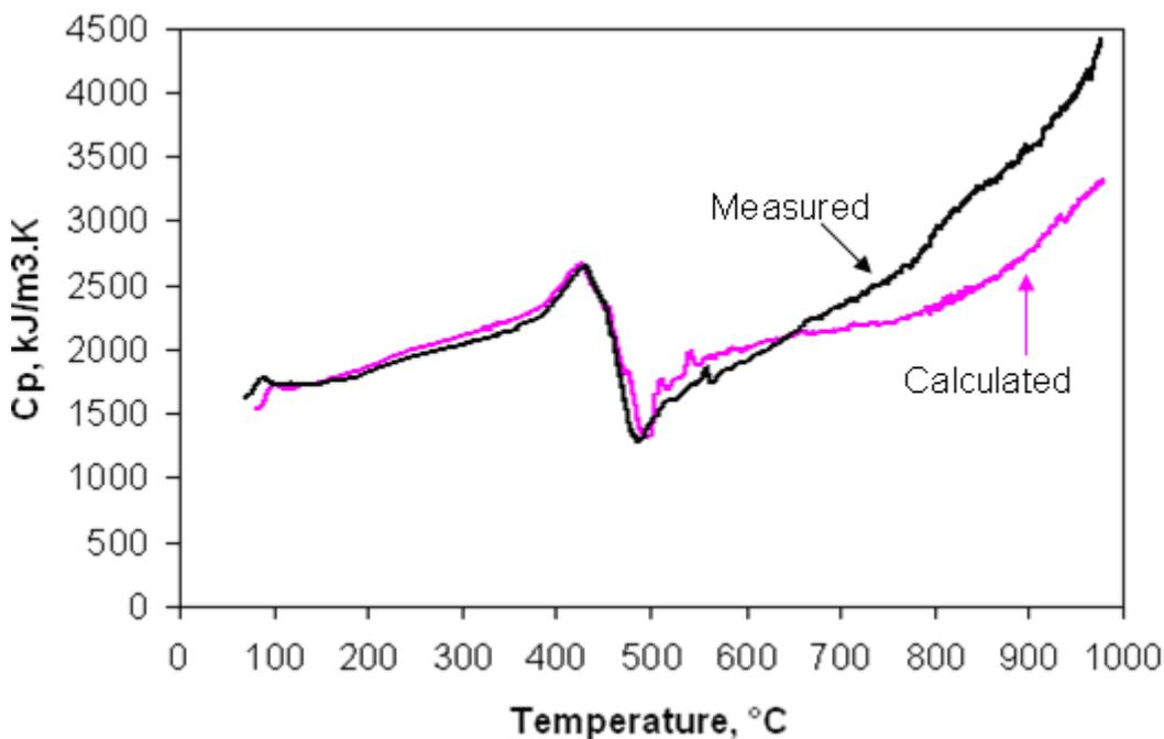
**Figure 6.12. Calculated by mass average and measured Cp for a blend of 85.4% vitrinite concentrate, with a particle size of 106-212  $\mu\text{m}$  and 85.7% vitrinite concentrate with a particle size of 212-500  $\mu\text{m}$ , bended at a ratio of 1:1 by mass, at a heating rate of 10°C/min from 25 to 1000°C.**
