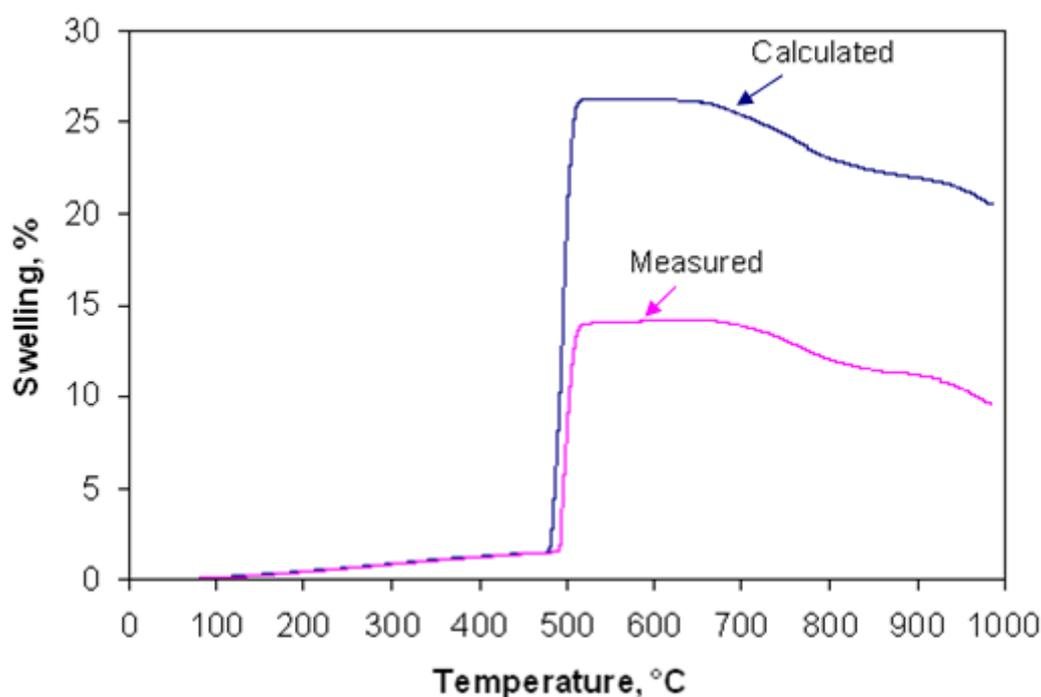
**Figure 5.8. Measured and calculated swelling results at a heating rate of 10°C/min from 25 to 1000°C for the blend made up of two vitrinite rich and one inertinite rich concentrates of b, d and f (81.8%, 81.6% and 29.0% vitrinite) at a ratio of 1:1:1 by mass.**
