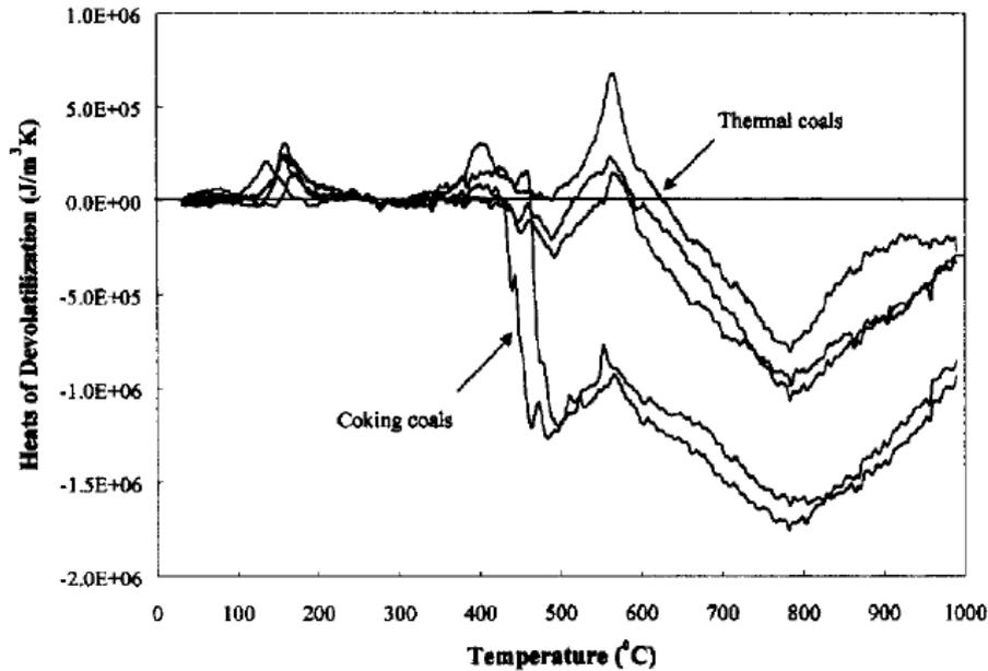
**Figure 2.15.** Heats of devolatilisation with temperature, calculated by subtracting the apparent specific heat from the real specific heat [21].
