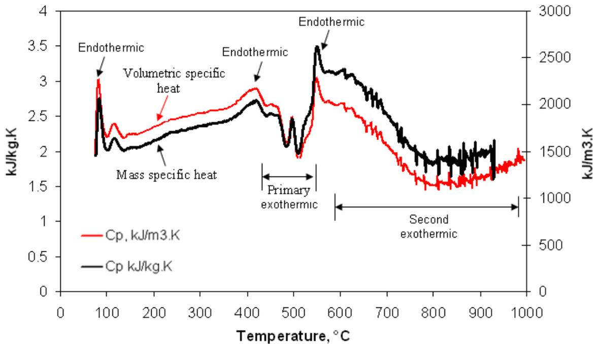
**Figure 4.4.** Comparison of the apparent volumetric specific heat and the apparent mass specific heat for coal sample C at a heating rate of 10°C/min from 25 to 1000°C.
