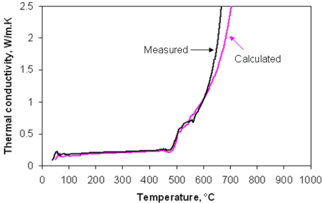
Figure 6.13. Calculated by mass average and measured thermal conductivity for a blend of 85.4% vitrinite concentrate with a particle size of 106-212  $\mu\text{m}$  and 85.7% vitrinite concentrate with a particle size of 212-500  $\mu\text{m}$  at a blending ratio of 1:1 by mass, at a heating rate of 10°C/min from 25 to 1000°C.
