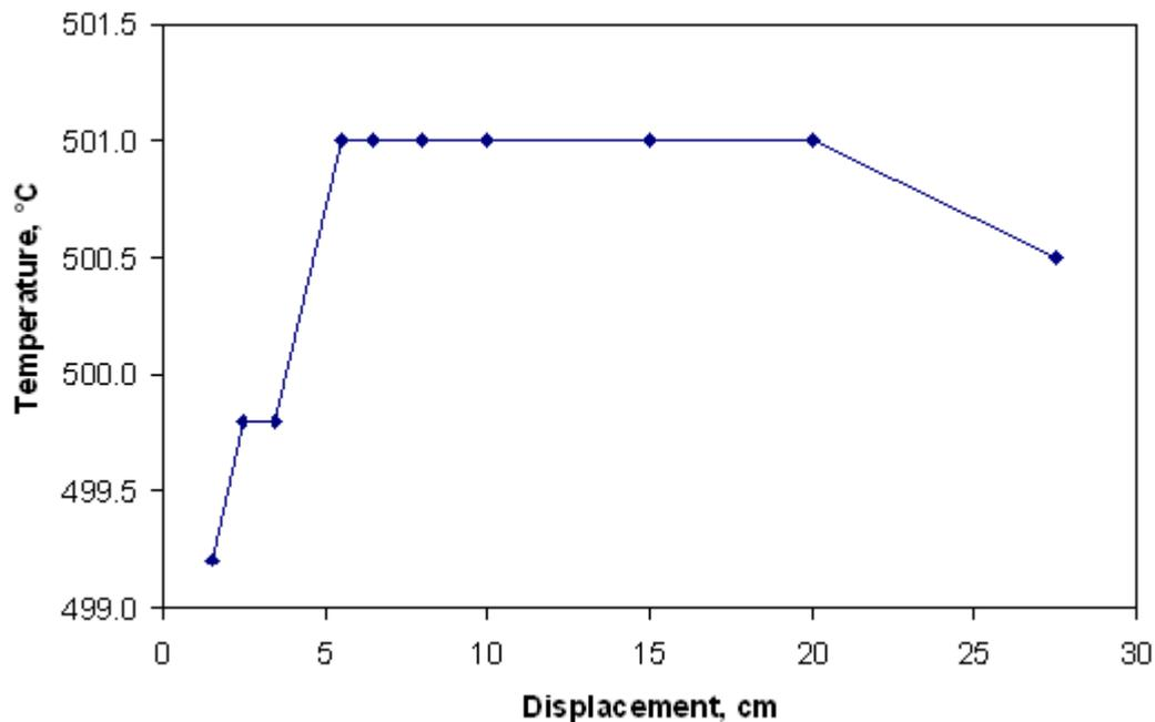
Figure A.1. Temperature distribution of the Sin-ku Riko Gold Image infrared heating furnace.
