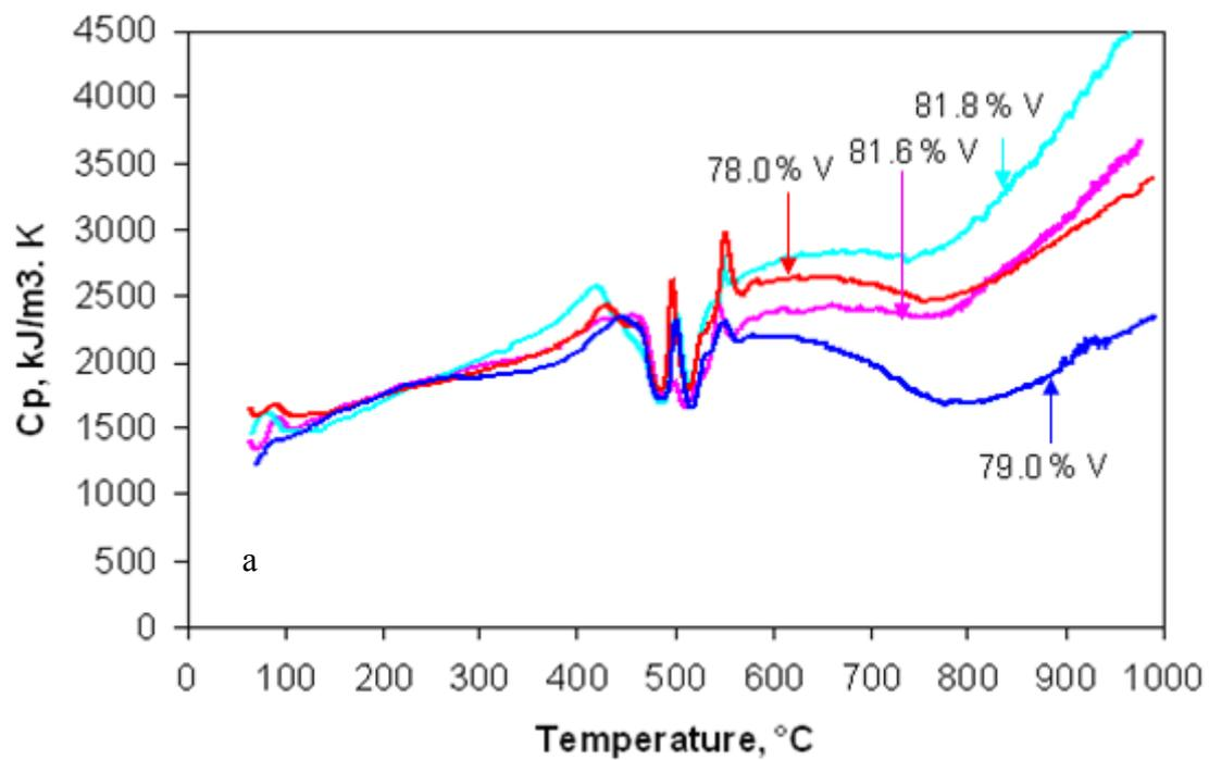
Figure 5.3 (a). Apparent specific heat of four vitrinite rich concentrates separated from the parent coal sample C at a heating rate of 10°C/min from 25 to 1000°C.
