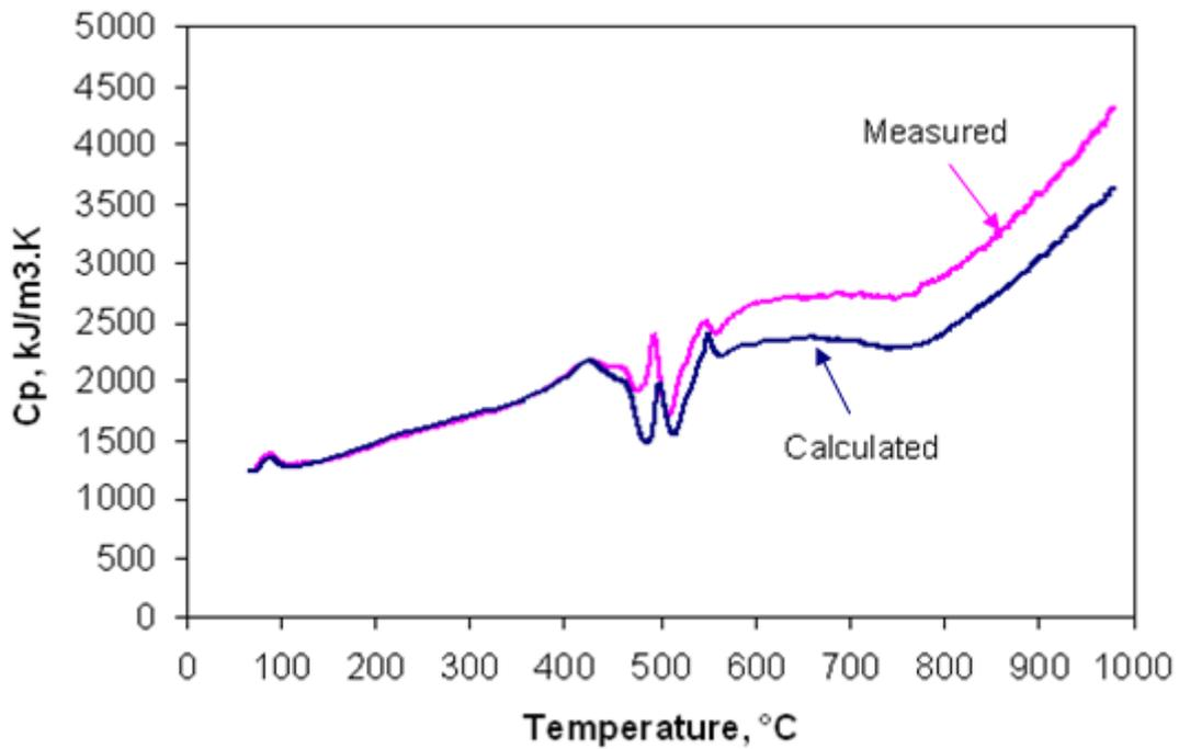
Figure 5.6. Measured and calculated apparent specific heat results at a heating rate of 10°C/min from 25 to 1000°C for the blend made up of three vitrinite rich concentrates of a, b and d (78.0%, 81.8% and 81.6% vitrinite) at a ratio of 1:1:1 by mass.
