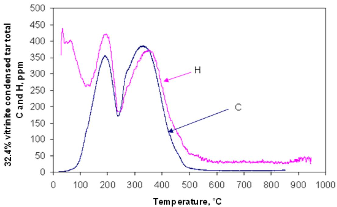
Figure 8.21. Properties of condensed tar obtained from the 32.4% vitrinite concentrate at a heating rate of 10°C/min from 25 to 1000°C.
