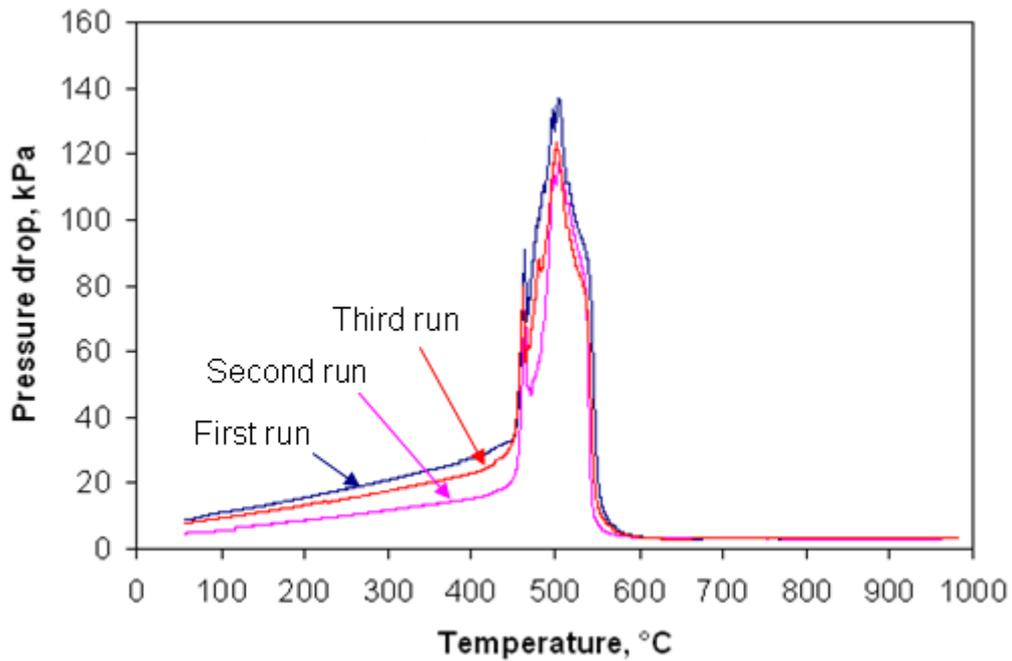
Figure 7.2. Pressure drop of the 86.4% vitrinite concentrate at a heating rate of 10°C/min from 25 to 1000°C for three replicate experiments.
