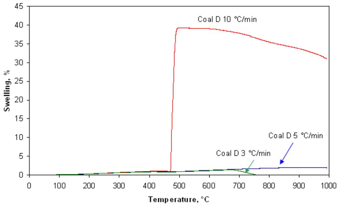
**Figure 4.10. Swelling of coal sample D at three different heating rates of 3, 5 and 10°C/min from 25 to 1000°C.**
