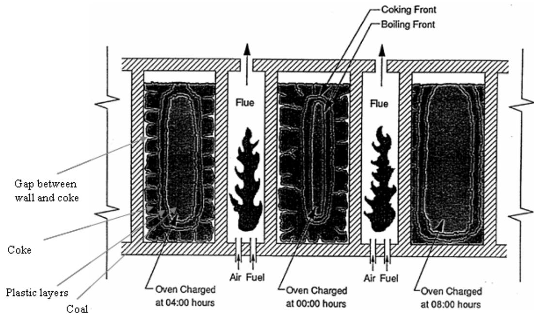
Figure 1.1. A longitudinal section of a coke oven battery [24].
