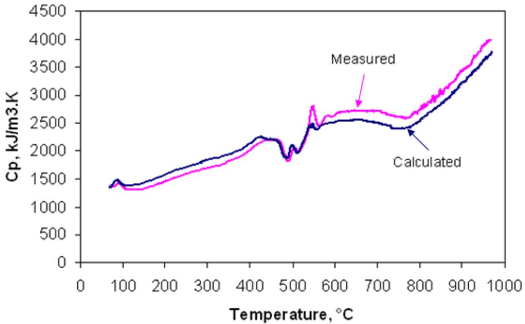
Figure 5.9. Measured and calculated apparent specific heat results at a heating rate of  $10^{\circ}\text{C}/\text{min}$  from 25 to  $1000^{\circ}\text{C}$  for the blend made up of two vitrinite rich and one inertinite rich concentrates of b, d and f (81.8%, 81.6% and 29.0% vitrinite) at a ratio of 1:1:1 by mass.
