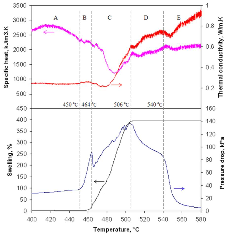
**Figure 7.6. Correlation between swelling, pressure drop of gas flowing through the coal sample, apparent specific heat and thermal conductivity for the 86.4% vitrinite concentrate at a heating rate of 10°C/min.**
