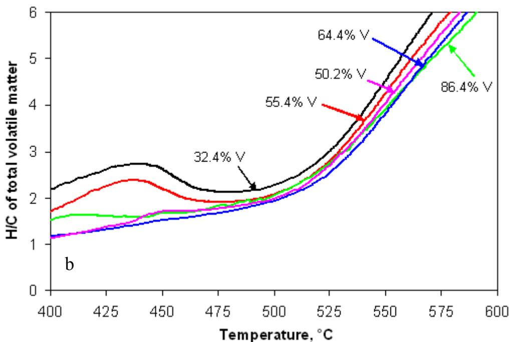
Figure 8.4 (b). A re-scaled H/C during the primary devolatilisation for Figure 8.4 (a).
