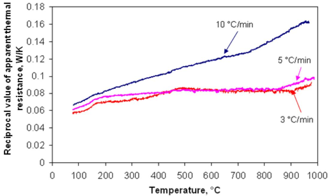
**Figure A.4. Reciprocal value of the apparent thermal resistance of heating furnace at three different heating rates calibrated by a copper.**
