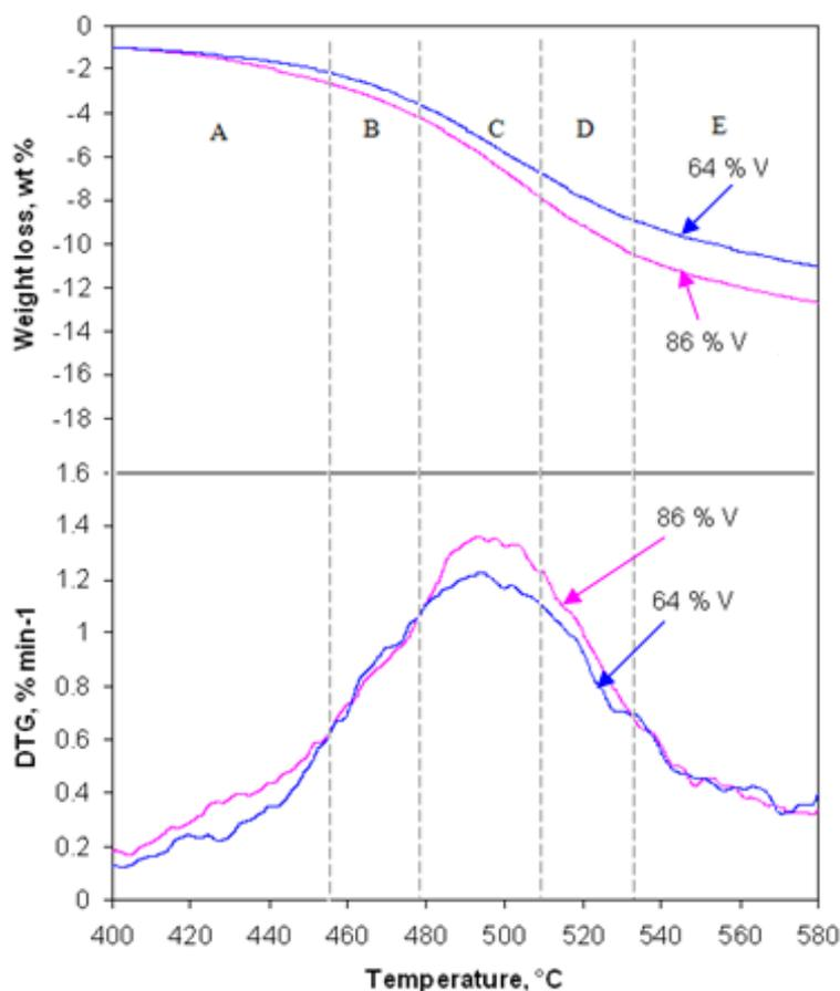
Figure 7.8. TG-DTG results for the 86.4% and 64.4% vitrinite concentrates at a heating rate of 10°C/min.
