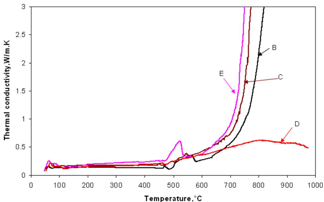
**Figure 4.5. Comparison of the thermal conductivities of the four coal samples at a heating of 10°C/min from 25 to 1000°C.**
