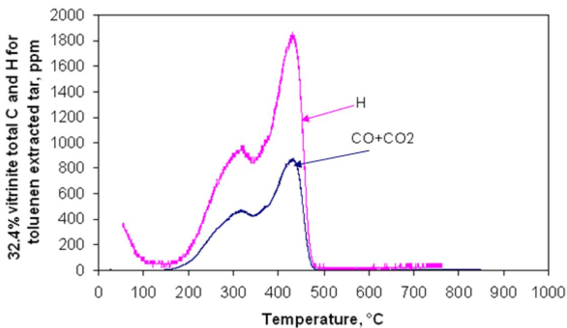
Figure 8.28. Properties of toluene extracted tar obtained from the 32.4% vitrinite concentrate at a heating rate of 10°C/min from 25 to 505°C.
