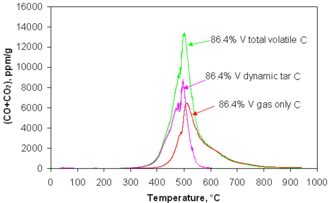
**Figure 8.6. Carbon concentration for total volatile, gas only and mathematically derived dynamic tar for the 86.4% vitrinite concentrate at a heating rate of 10°C/min from 25 to 1000°C.**
