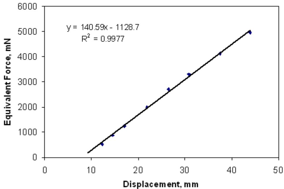
Figure A.2. Relationship between spring compression and equivalent force.
