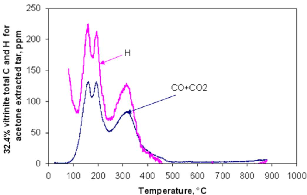
Figure 8.26. Properties of acetone extracted tar obtained from the 32.4% vitrinite concentrate at a heating rate of 10°C/min from 25 to 505°C.
