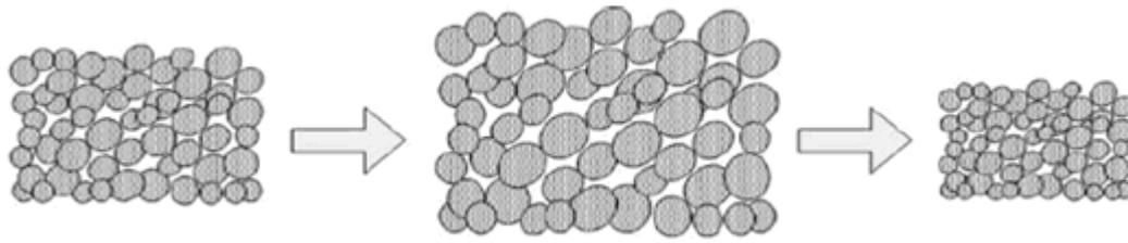
**Figure 2.11. Schematic diagram of the swelling and shrinkage of coal during pyrolysis [111].**
