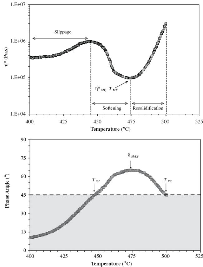
Figure 2.6. (Top)  $\eta^*$  as a function of temperature for one heating coking coal (71% vitrinite), (bottom) phase angle ( $\delta$ ) as a function of temperature for the same heating coal [88].
