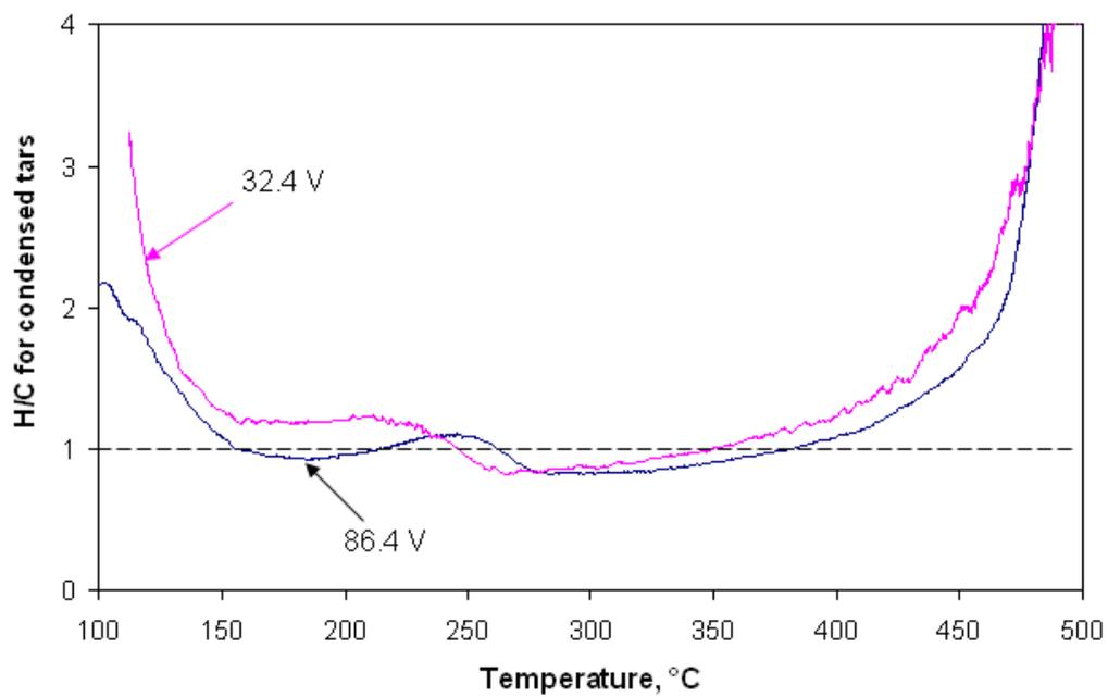
**Figure 8.22** H/C for condensed tar obtained from the 86.4% and 32.4% vitrinite concentrates at a heating rate of 10°C/min from 25 to 1000°C.
