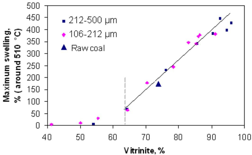
Figure 6.14. Relationship between vitrinite content and maximum swelling (at about 510°C) for the 106-212 μm and 212-500 μm size cuts of coal maceral concentrates at a heating rate of 10°C/min.
