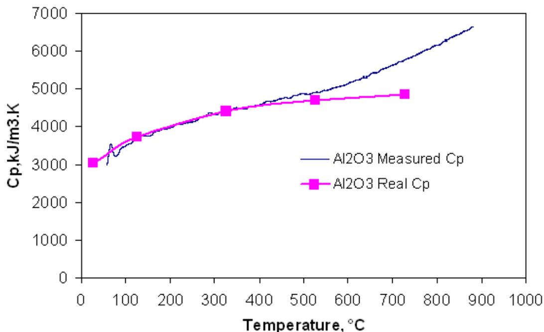
Figure A.5. Calculated Cp comparing to real Cp of Al<sub>2</sub>O<sub>3</sub> at a heating rate of 10°C/min.
