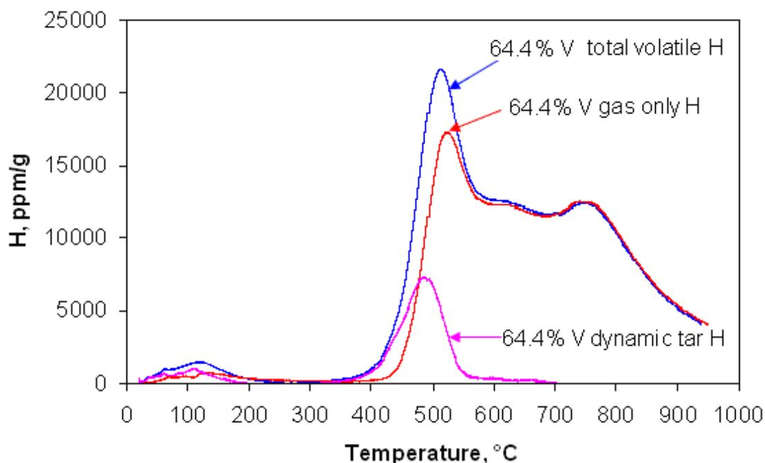
Figure 8.7. Hydrogen concentration for total volatile, gas only and mathematically derived dynamic tar for the 64.4% vitrinite concentrate at a heating rate of 10°C/min from 25 to 1000°C.
