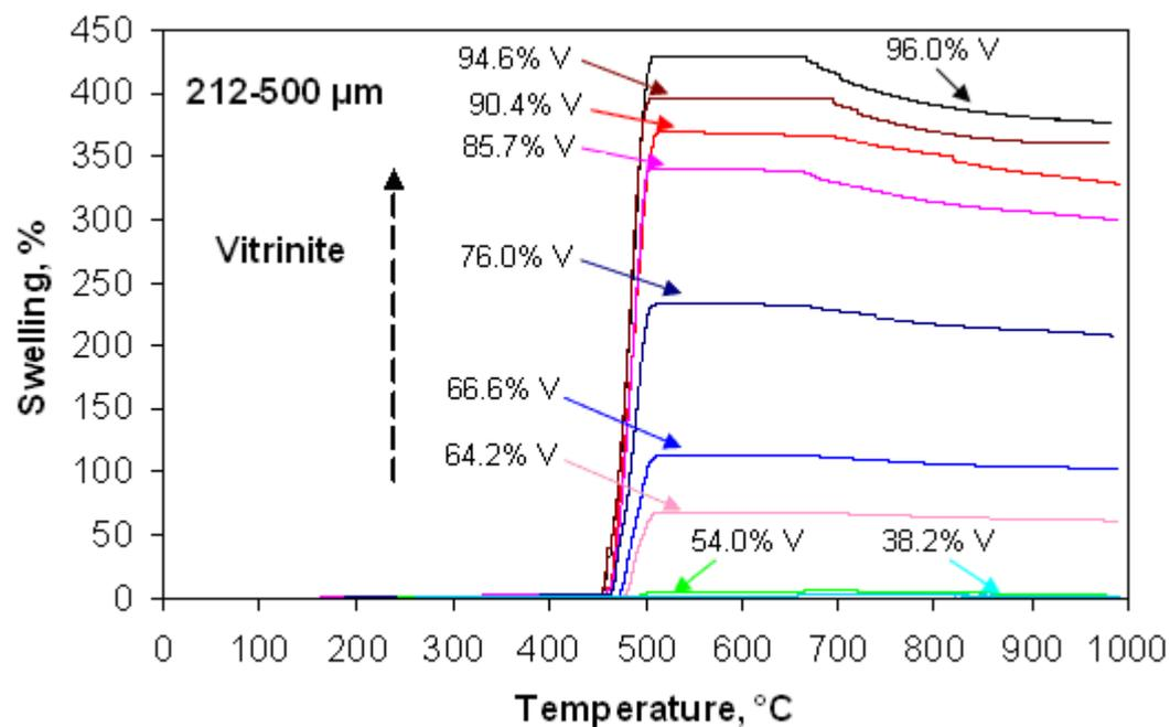
Figure 6.4. Swelling for 212-500  $\mu\text{m}$  coal maceral concentrates at a heating rate of 10°C/min from 25 to 1000°C.
