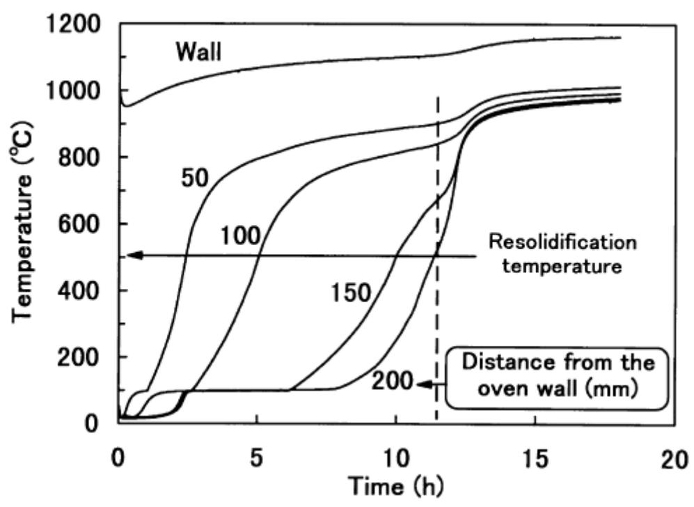
Figure 1.2. Changes in temperature with time at the relevant distance from the oven wall [25].
