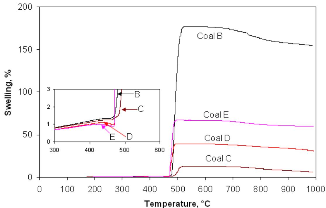
Figure 4.1. Swelling of four coal samples at a heating rate of 10°C/min from 25 to 1000°C.
