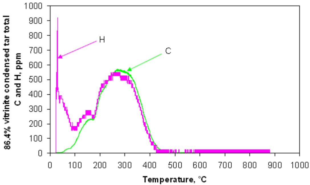
Figure 8.23. Properties of condensed tar obtained from the 86.4% vitrinite concentrate at a heating rate of 10°C/min from 25 to 505°C.
