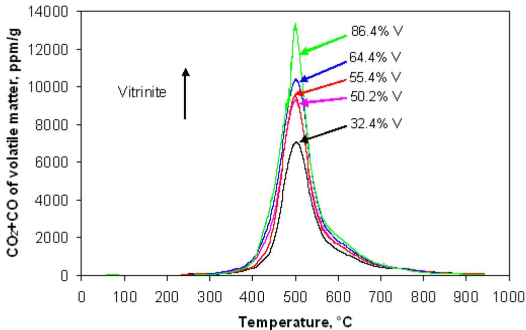
Figure 8.3. Carbon concentration of total volatiles for various coal maceral concentrates at a heating rate of 10°C/min from 25 to 1000°C.
