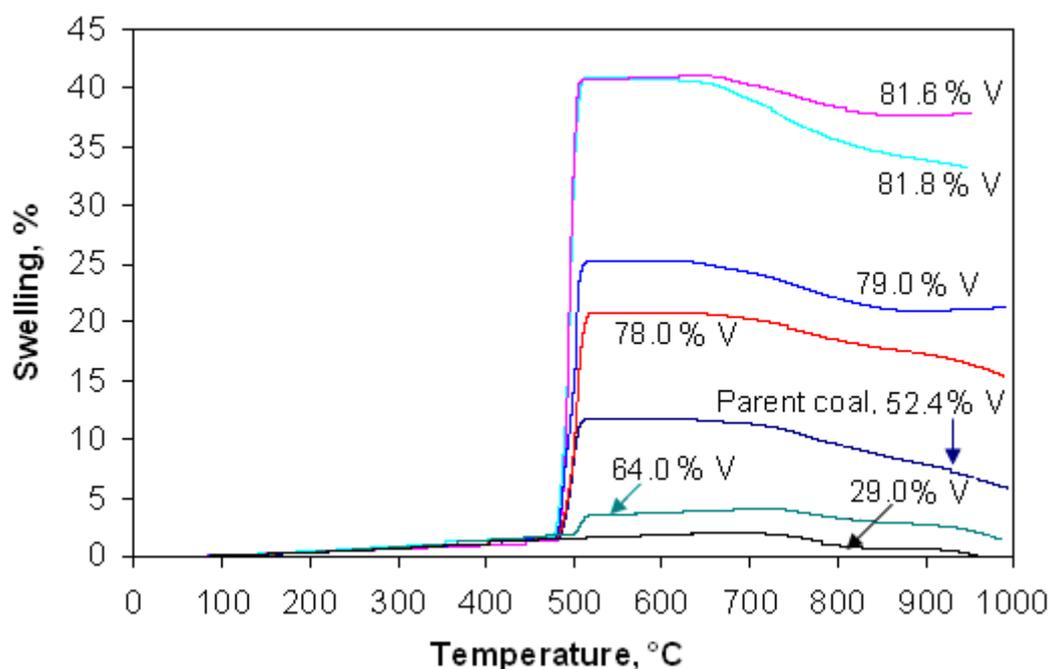
**Figure 5.2.** Swelling behaviour of coal sample C and coal maceral concentrates separated from parent coal sample C at a heating rate of 10°C/min from 25 to 1000°C.
