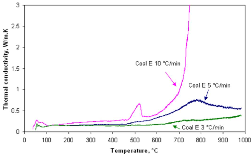
Figure 4.20. Thermal conductivities of coal sample E at three different heating rates of 3, 5 and 10°C/min from 25 to 1000°C.
