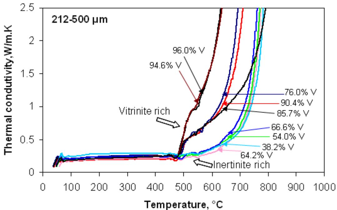
**Figure 6.8.** Thermal conductivity for 212-500  $\mu\text{m}$  coal maceral concentrates at a heating rate of  $10^\circ\text{C}/\text{min}$  from 25 to  $1000^\circ\text{C}$ .
