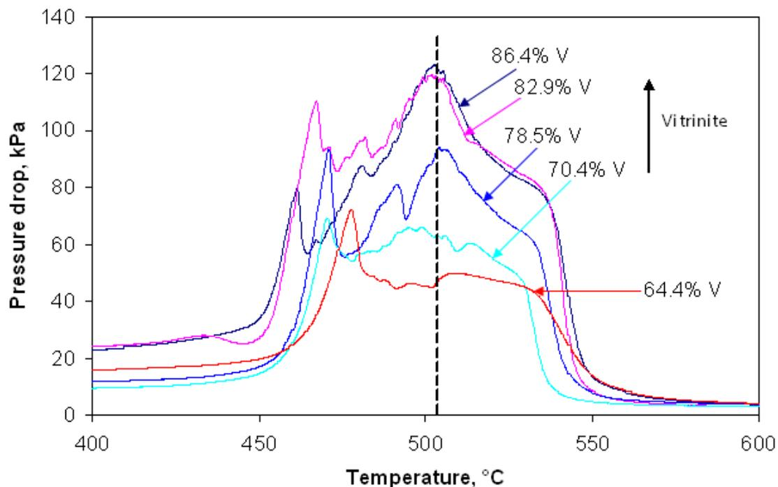
Figure 7.9. Pressure drop of gas flowing through the coal maceral concentrates at a heating rate of 10°C/min.
