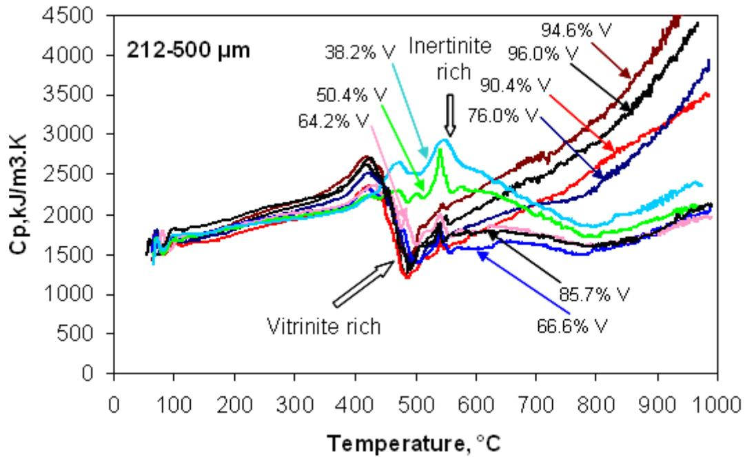
Figure 6.6. Apparent specific heat for 212-500  $\mu\text{m}$  coal maceral concentrates at a heating rate of  $10^\circ\text{C}/\text{min}$  from 25 to  $1000^\circ\text{C}$ .
