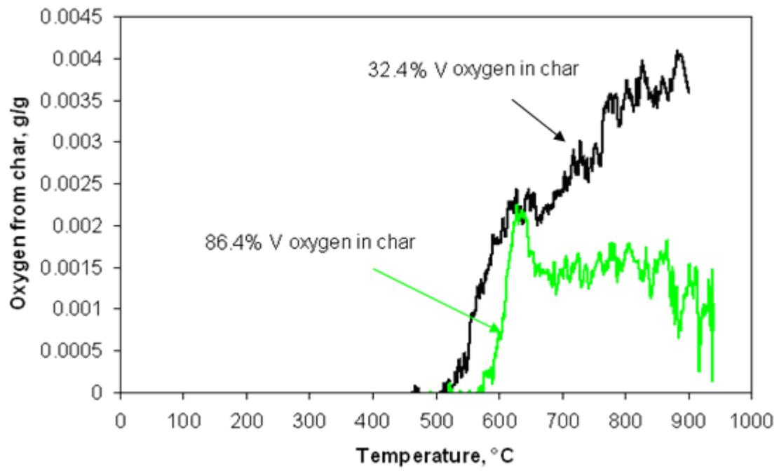
Figure 8.18. Oxygen released from chars for the 86.4% and 32.4% vitrinite concentrates at a heating rate of 10°C/min from 25 to 1000°C.
