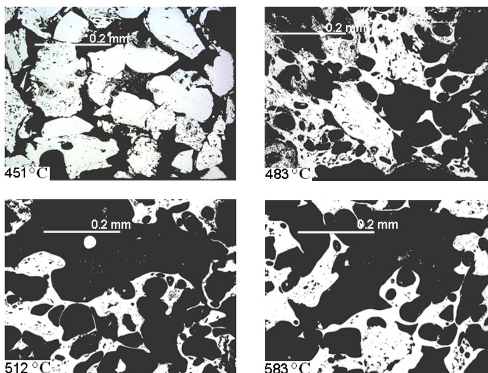
Figure 7.12. Optical microscopy images for the 64.4% vitrinite concentrate quenched at critical temperature points.
