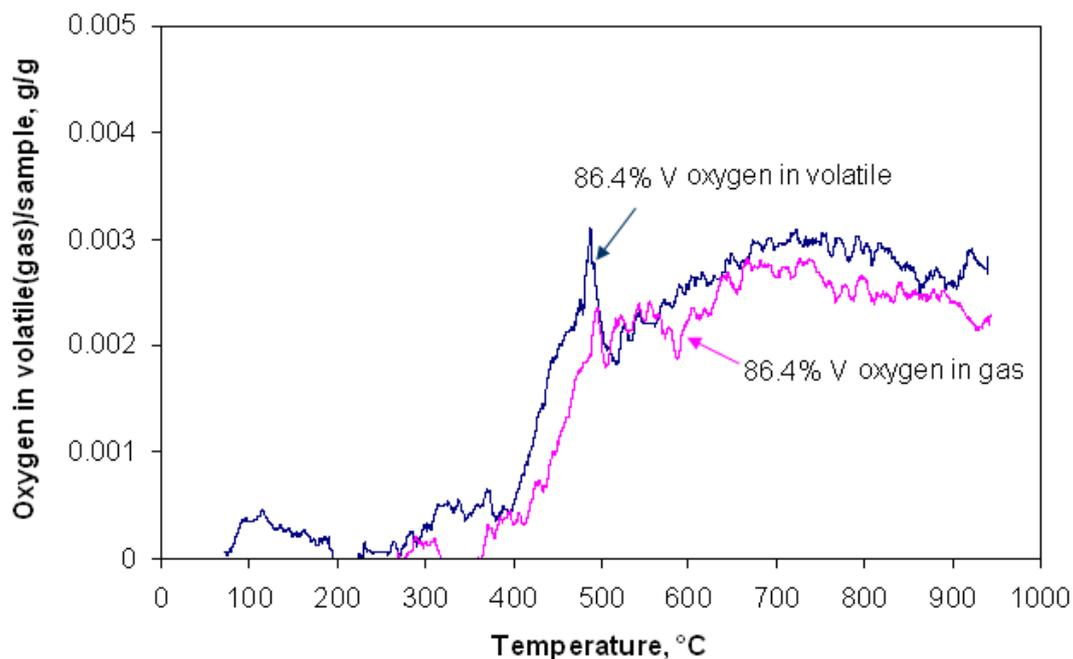
**Figure 8.14. Oxygen in volatile matter and gas only for the 86.4% vitrinite concentrate at a heating rate of 10°C/min from 25 to 1000°C.**
