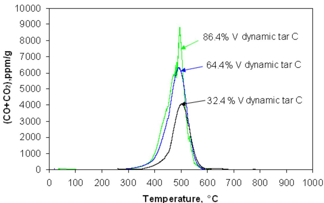
**Figure 8.12. Comparison of C for mathematically derived dynamic tar for the 86.4%, 64.4% and 32.4% vitrinite concentrates at a heating rate of 10°C/min from 25 to 1000°C.**
