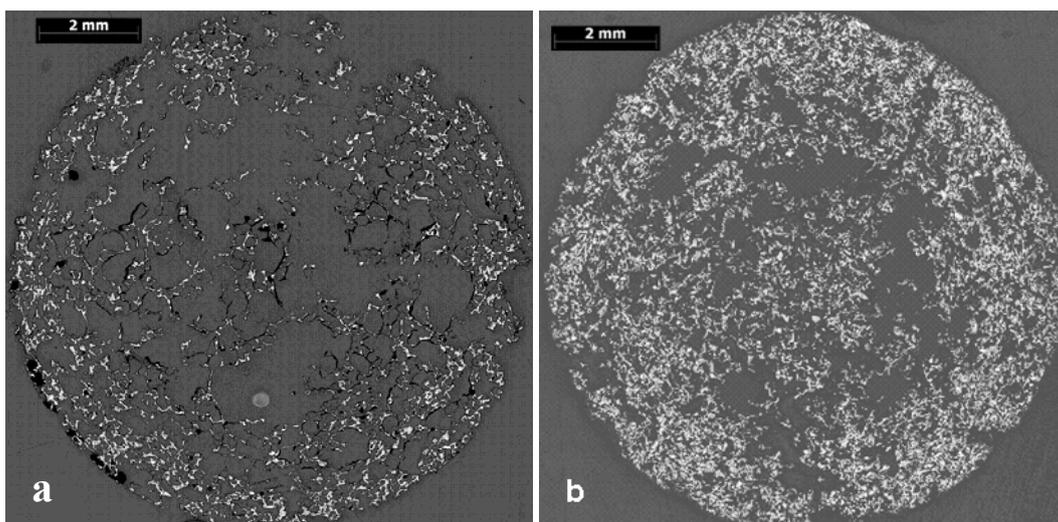
**Figure 6.10.** Optical microscopy overview images of the cross section of the cylindrical coke obtained from 106-212  $\mu\text{m}$  (a) 86.4% vitrinite concentrate, (b) 64.4% vitrinite concentrate at a heating rate of  $10^\circ\text{C}/\text{min}$  from 25 to  $1000^\circ\text{C}$ .
