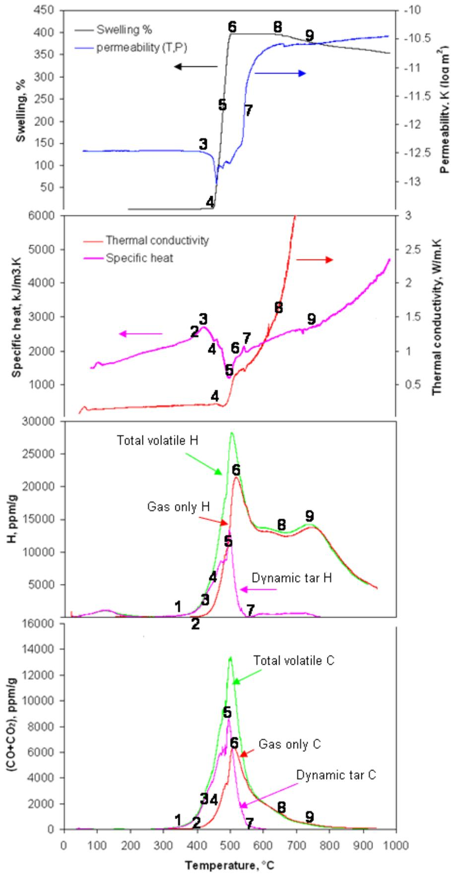
Figure 9.1. Correlations of physical, chemical and thermal changes during coke formation for the 86.4% vitrinite concentrate.
