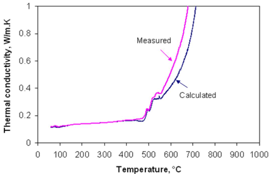
Figure 5.7. Measured and calculated thermal conductivity results at a heating rate of 10°C/min from 25 to 1000°C for the blend made up of three vitrinite rich concentrates of a, b and d (78.0%, 81.8% and 81.6% vitrinite) at a ratio of 1:1:1 by mass.
