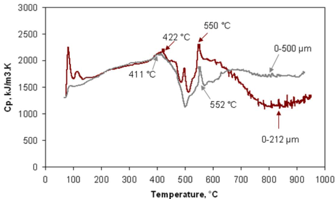
**Figure 4.23. Effect of particles size on the apparent specific heat for coal sample C at a heating rate of 10°C/min from 25 to 1000°C.**
