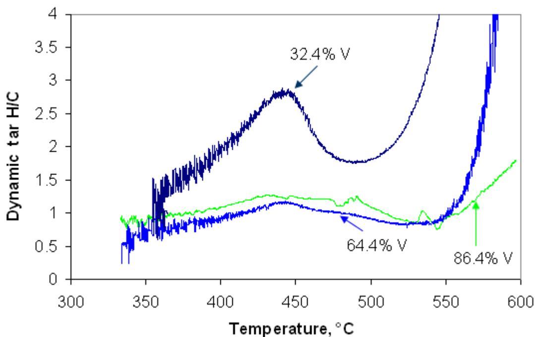
**Figure 8.13. Comparison of H/C for mathematically derived dynamic tar for the 86.4%, 64.4% and 32.4% vitrinite concentrates at a heating rate of 10°C/min from 25 to 1000°C.**
