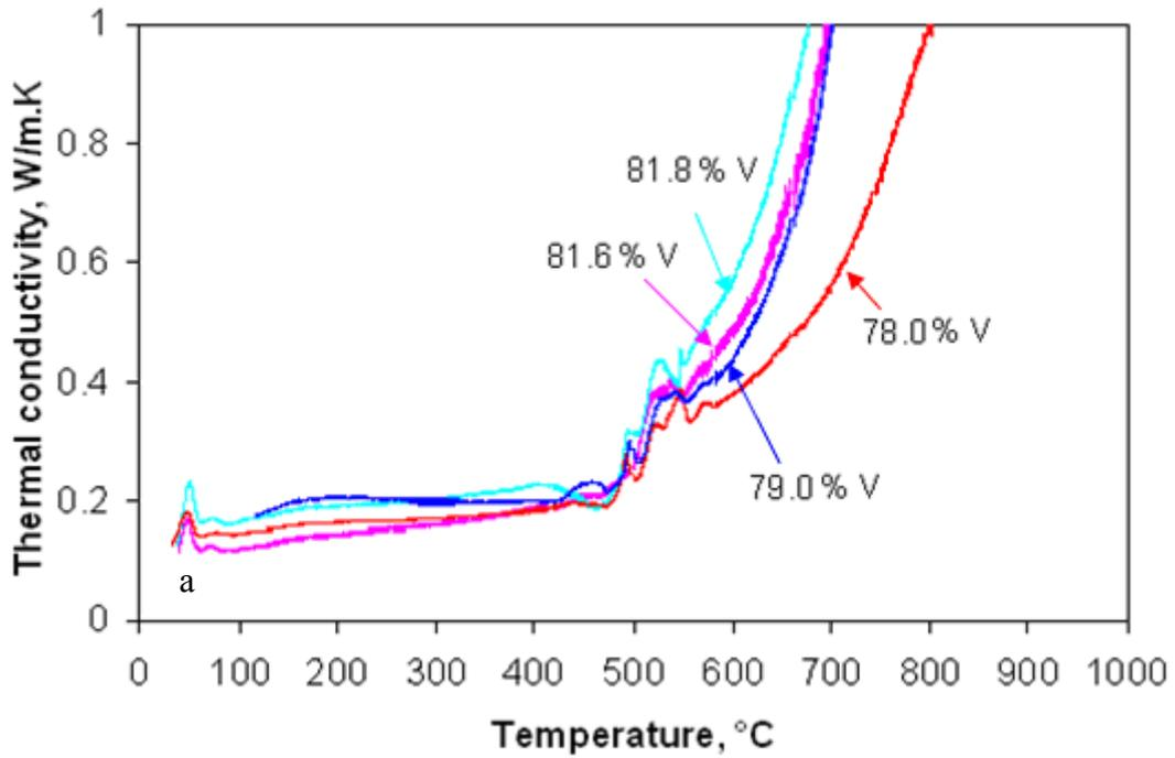
Figure 5.4 (a). Thermal conductivity of four vitrinite rich concentrates separated from the parent coal C at a heating rate of 10°C/min from 25 to 1000°C.
