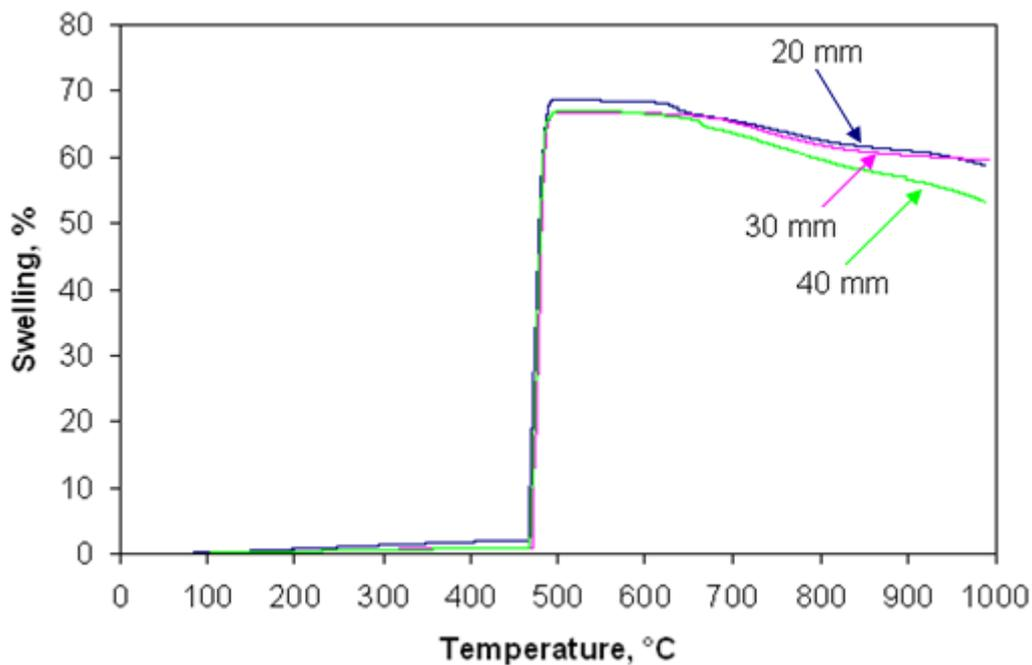
Figure B.1. Swelling of coal sample E at a heating rate of 10°C/min with different coal bed lengths.
