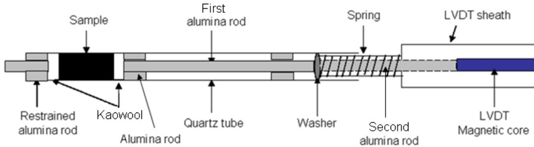
**Figure 3.3. Schematic representation for measuring swelling of heating coal and coal maceral concentrates.**
