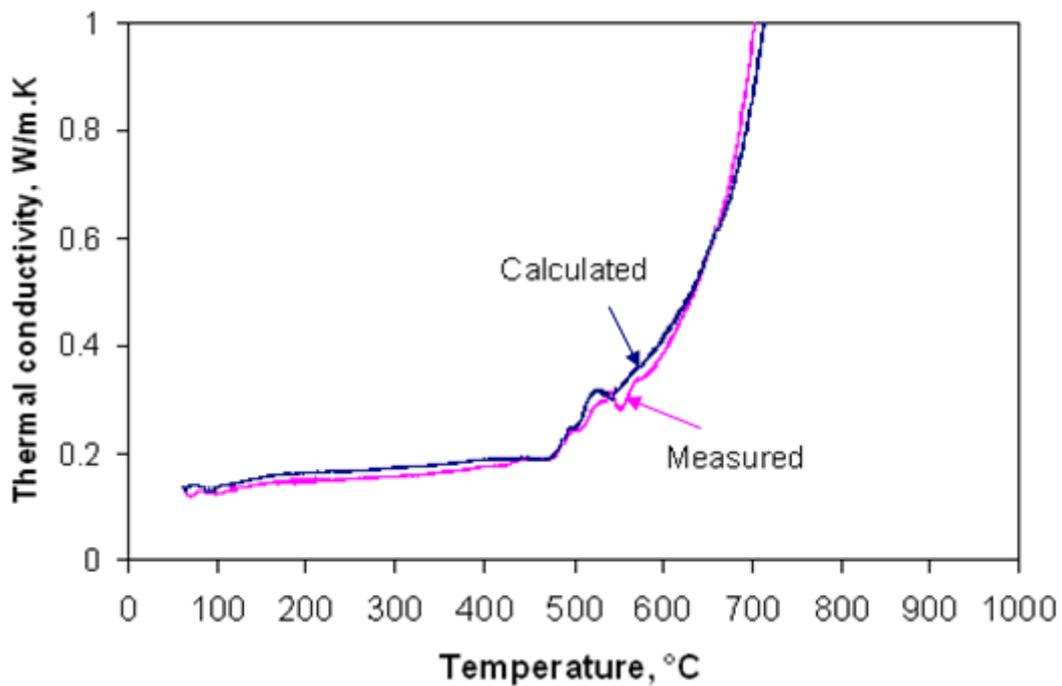
Figure 5.10. Measured and calculated thermal conductivity results at a heating rate of  $10^{\circ}\text{C}/\text{min}$  from 25 to  $1000^{\circ}\text{C}$  for the blend made up of two vitrinite rich and one inertinite rich concentrates of b, d and f (81.8%, 81.6% and 29.0% vitrinite) at a ratio of 1:1:1 by mass.
