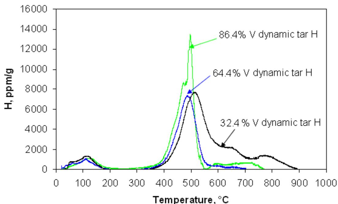
**Figure 8.11.** Comparison of H for mathematically derived dynamic tar for the 86.4%, 64.4% and 32.4% vitrinite concentrates at a heating rate of 10°C/min from 25 to 1000°C.
