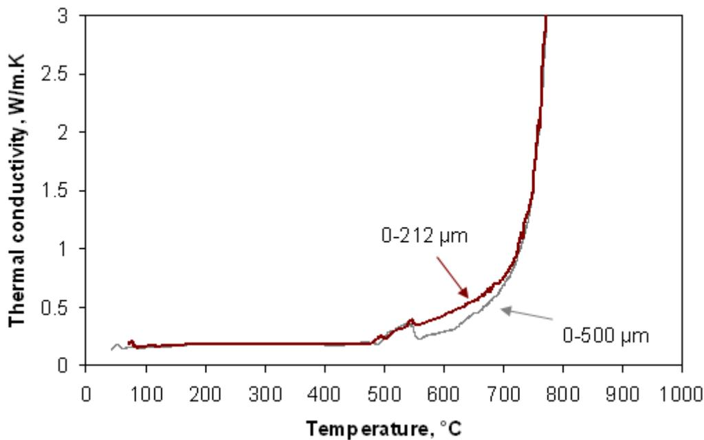
**Figure 4.24. Effect of particles size on the thermal conductivity for coal sample C at a heating rate of 10°C/min from 25 to 1000°C.**
