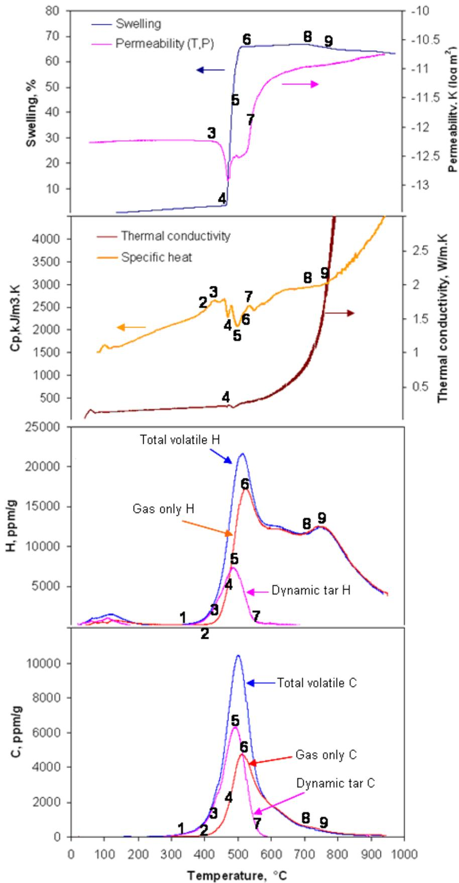
Figure 9.2. Correlations of physical, chemical and thermal changes during coke formation for the 64.4% vitrinite concentrate.
