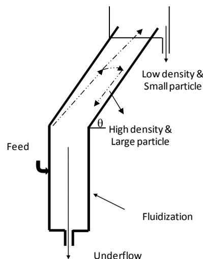
**Figure 3.1. Schematic representation of the reflux classifier showing the feed and a fluidized bed housing, 24 parallel channels in the inclined equipment were not directly presented.**
