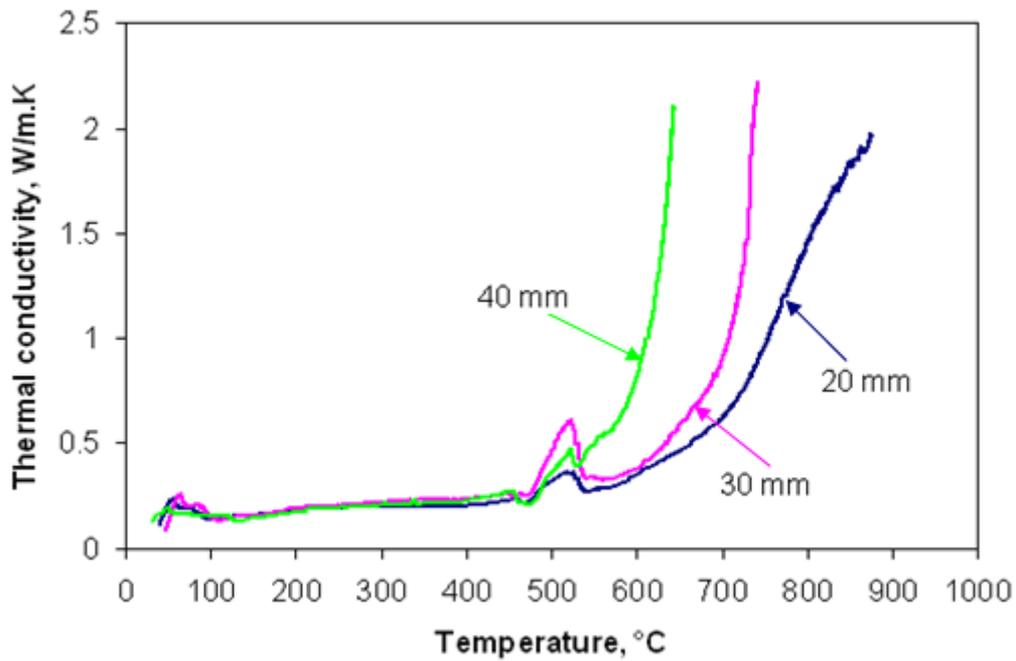
Figure B.3. Thermal conductivity of coal sample E at a heating rate of 10°C/min with different coal bed lengths.
