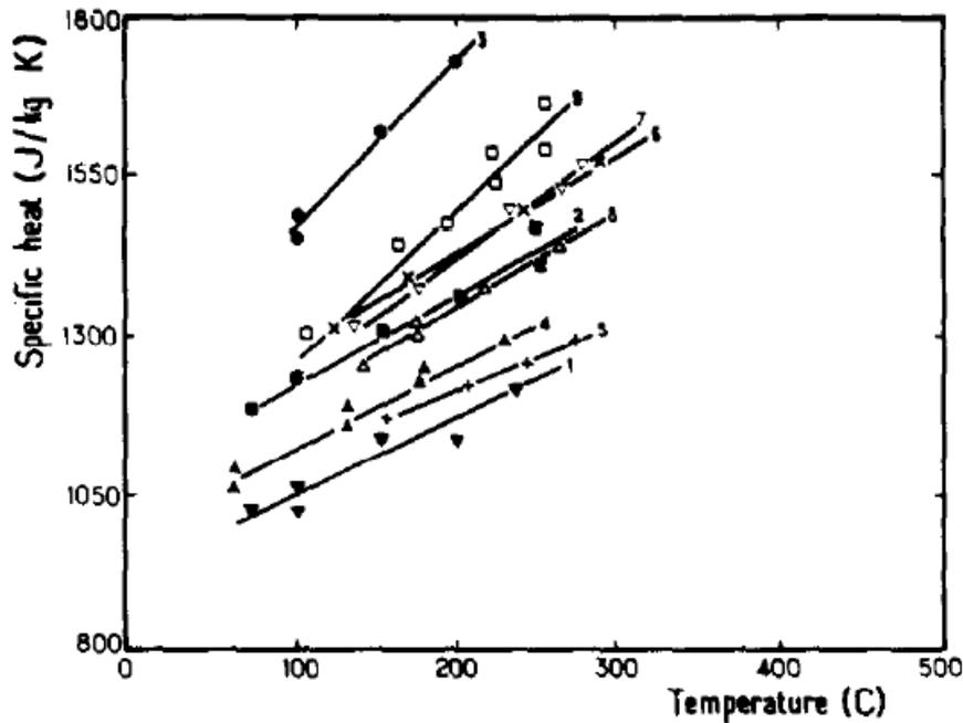
Figure 2.14. Mean specific heat of coal versus temperature [160].
