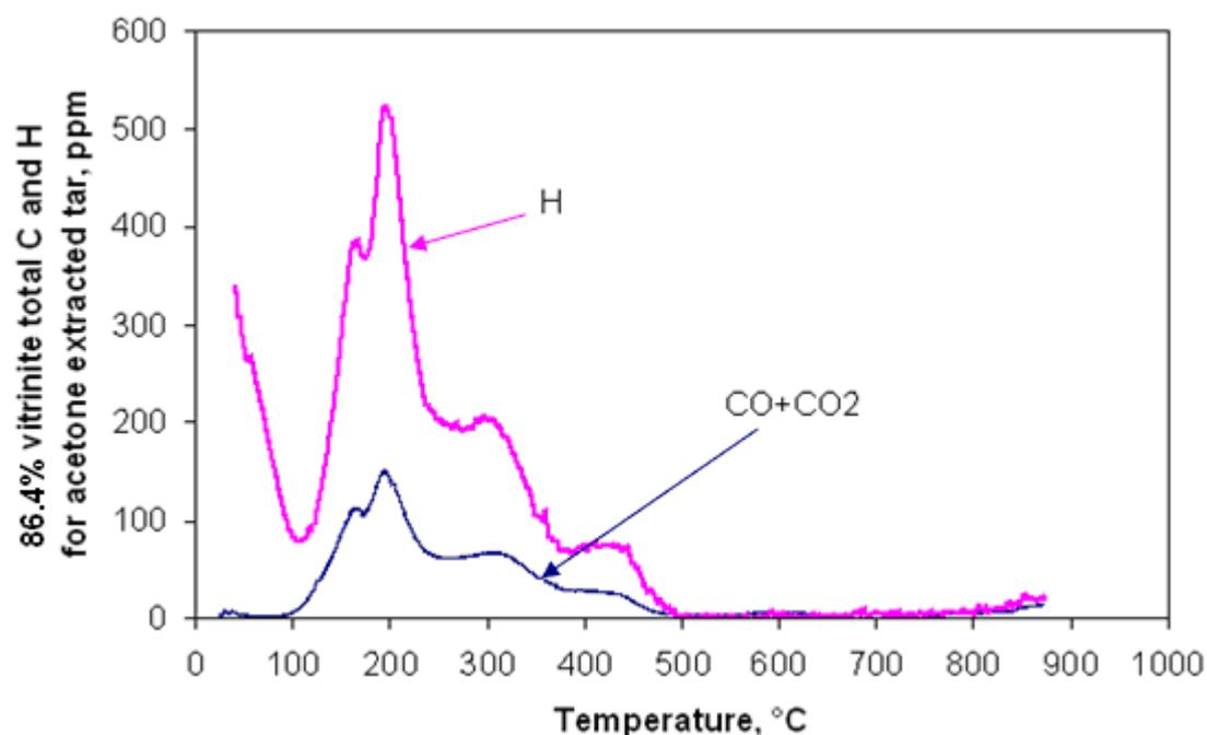
Figure 8.25. Properties of acetone extracted tar obtained from the 86.4% vitrinite concentrate at a heating rate of 10°C/min from 25 to 505°C.
