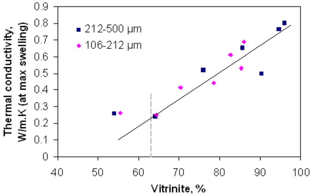
**Figure 6.20. Relationship between the thermal conductivity at the maximum swelling (at about 510°C) and the vitrinite content for the 106-212 μm and 212-500 μm size cuts of coal maceral concentrates at a heating rate of 10°C/min.**
