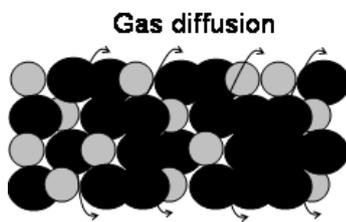
(b) Gas flow (mainly carrier gas and some volatiles) is hindered by a packed bed of solids and softening particles (280-400°C).
