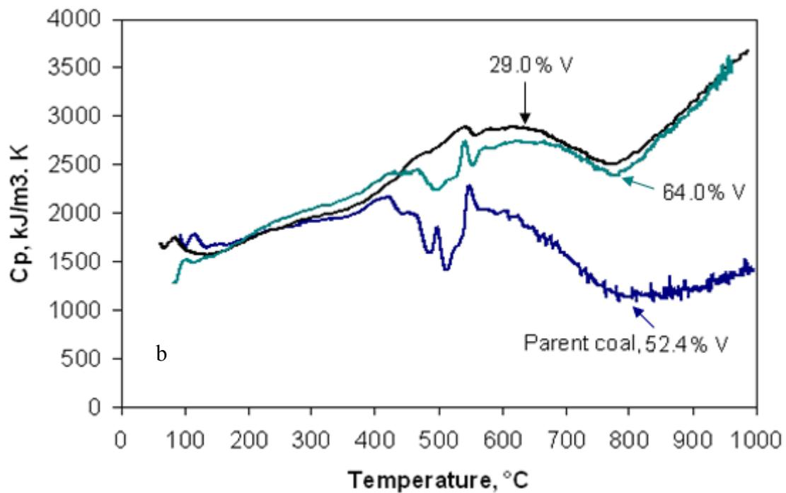
Figure 5.3 (b). Apparent specific heat of the parent coal C and two inertinite rich concentrates separated from the parent coal C at a heating rate of 10°C/min from 25 to 1000°C.
