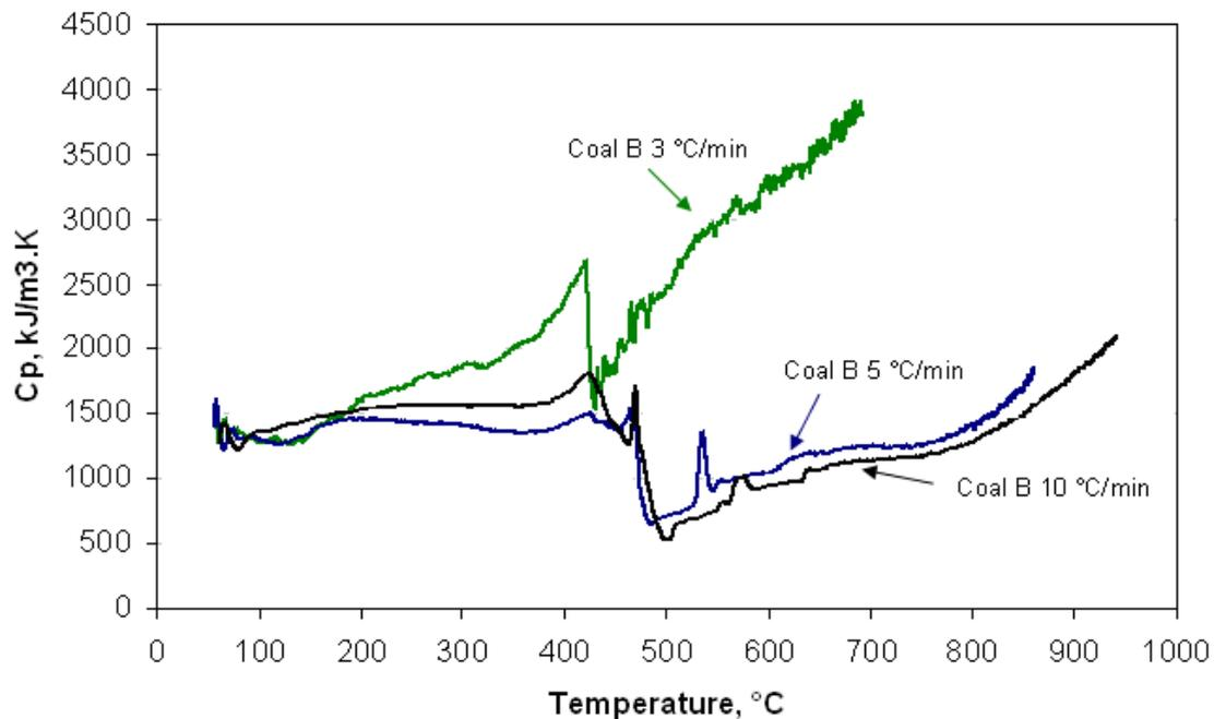
**Figure 4.13. Apparent specific heat of coal sample B at three different heating rates of 3, 5 and 10°C/min from 25 to 1000°C.**
