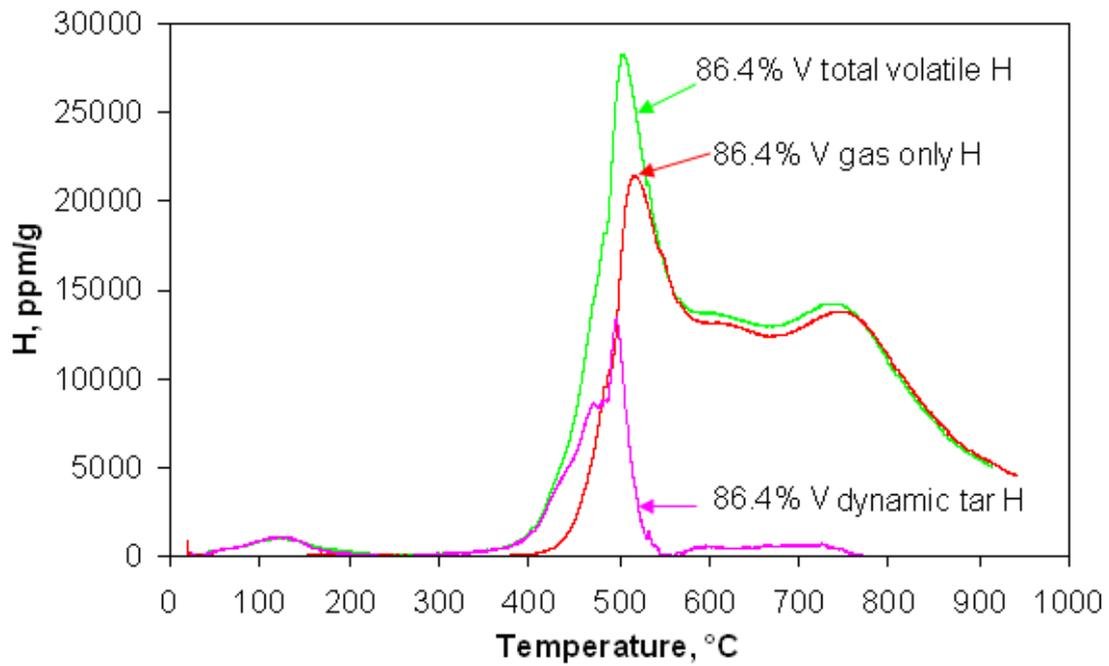
**Figure 8.5. Hydrogen concentration for total volatile, gas only and mathematically derived dynamic tar for the 86.4% vitrinite concentrate at a heating rate of 10°C/min from 25 to 1000°C.**
