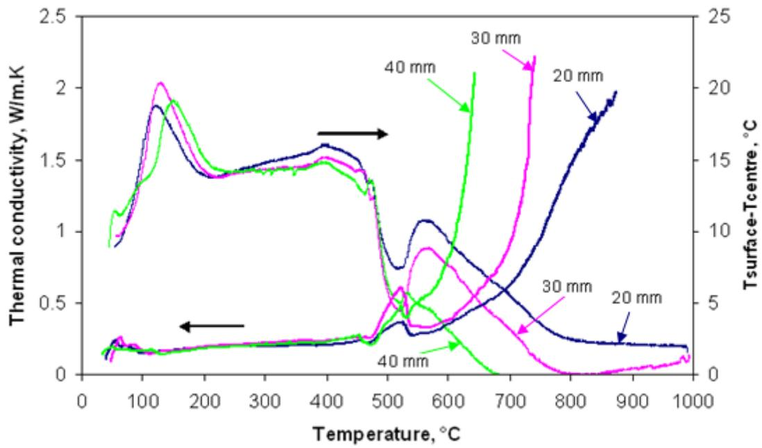
Figure B.5. The relationship between thermal conductivity and ( $T_{\text{surface}}-T_{\text{centre}}$ ) with different packed lengths under same heating conditions for coal sample E.
