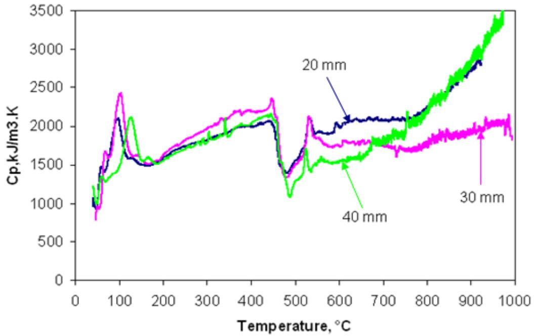
Figure B.2. Specific heat of coal sample E at a heating rate of 10°C/min with different coal bed lengths.
