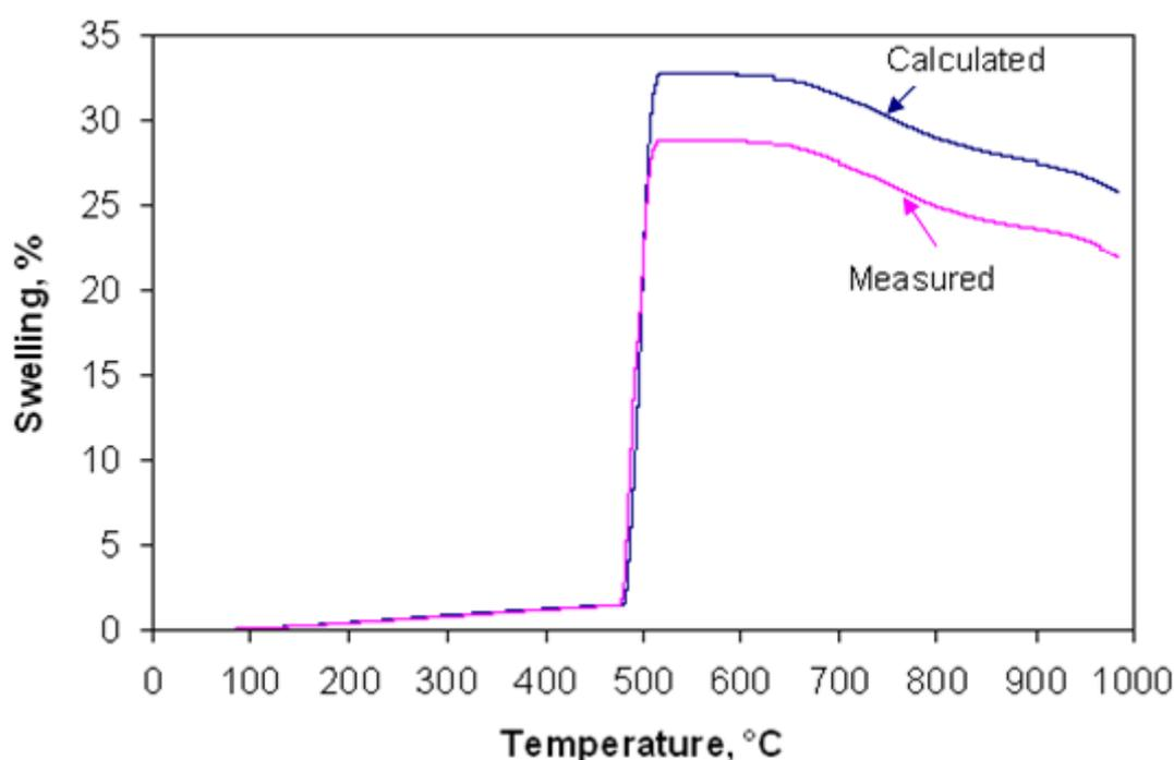
Figure 5.5. Measured and calculated swelling results at a heating rate of 10°C/min from 25 to 1000°C for the blend made up of three vitrinite rich concentrates of a, b and d (78.0%, 81.8% and 81.6% vitrinite) at a ratio of 1:1:1 by mass.
