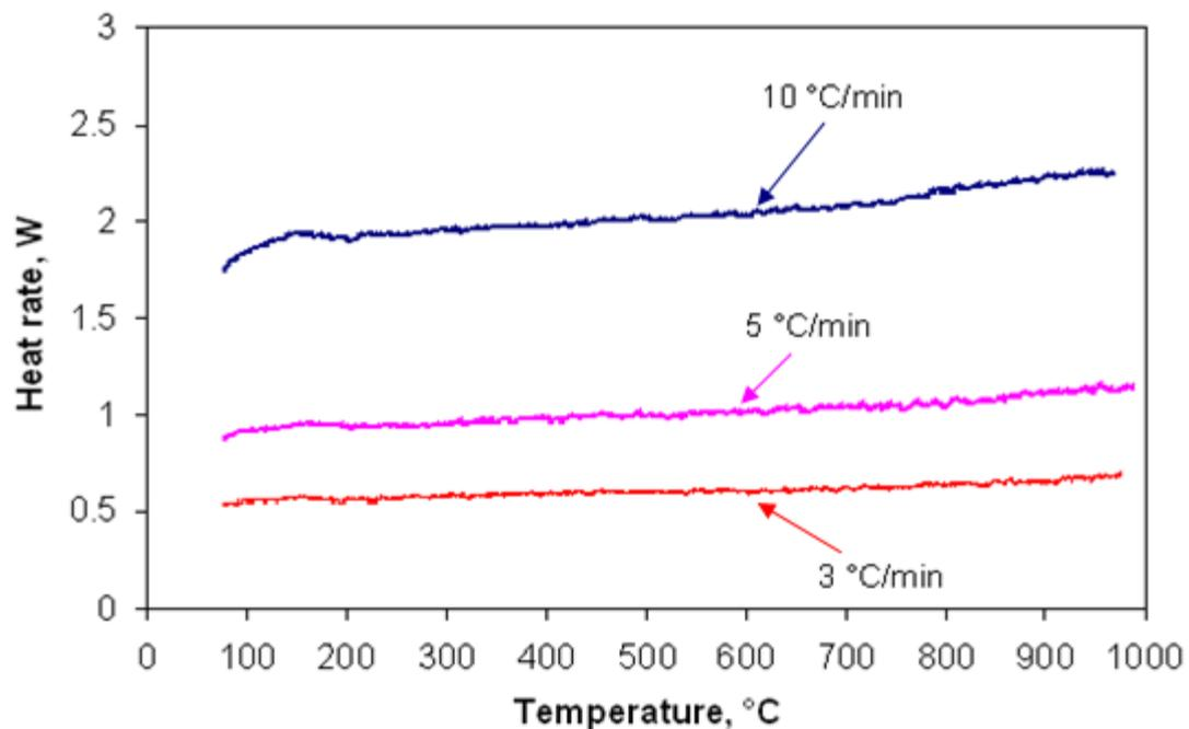
Figure A.3. Heat rate of heating furnace at three different heating rates calibrated by a copper.
