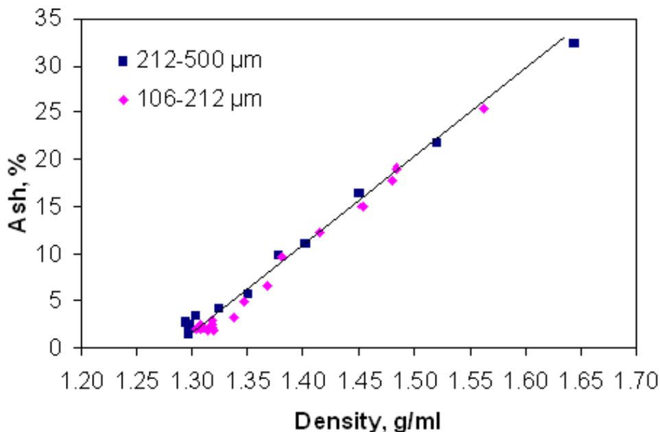
Figure 6.3. Relationship between density and ash content for all 106-212  $\mu\text{m}$  and 212-500  $\mu\text{m}$  size cuts of coal maceral concentrates.
