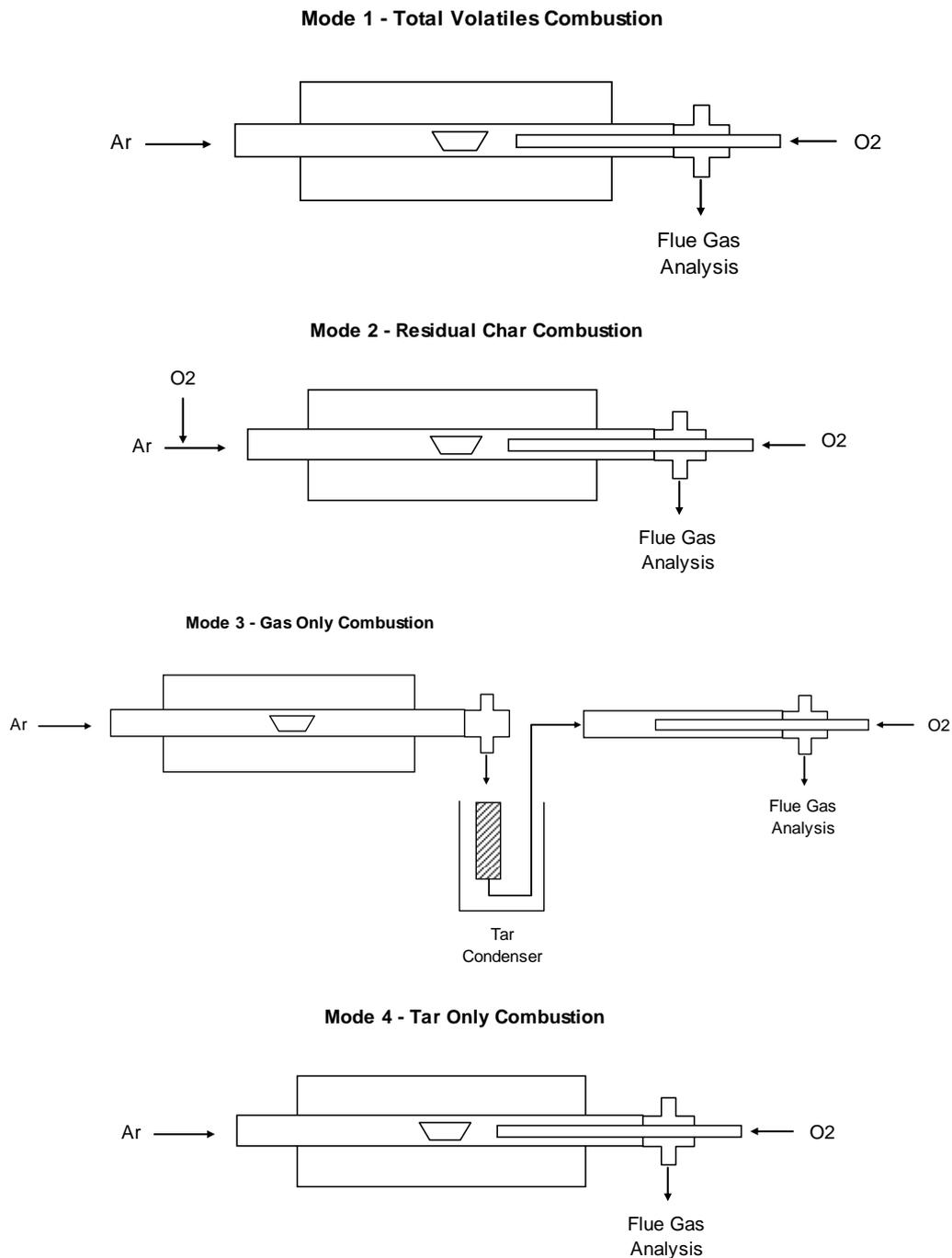
**Figure 3.5. Modes of operation using the DETA apparatus for analysing tars plus gases, char, gases only and tars only.**
