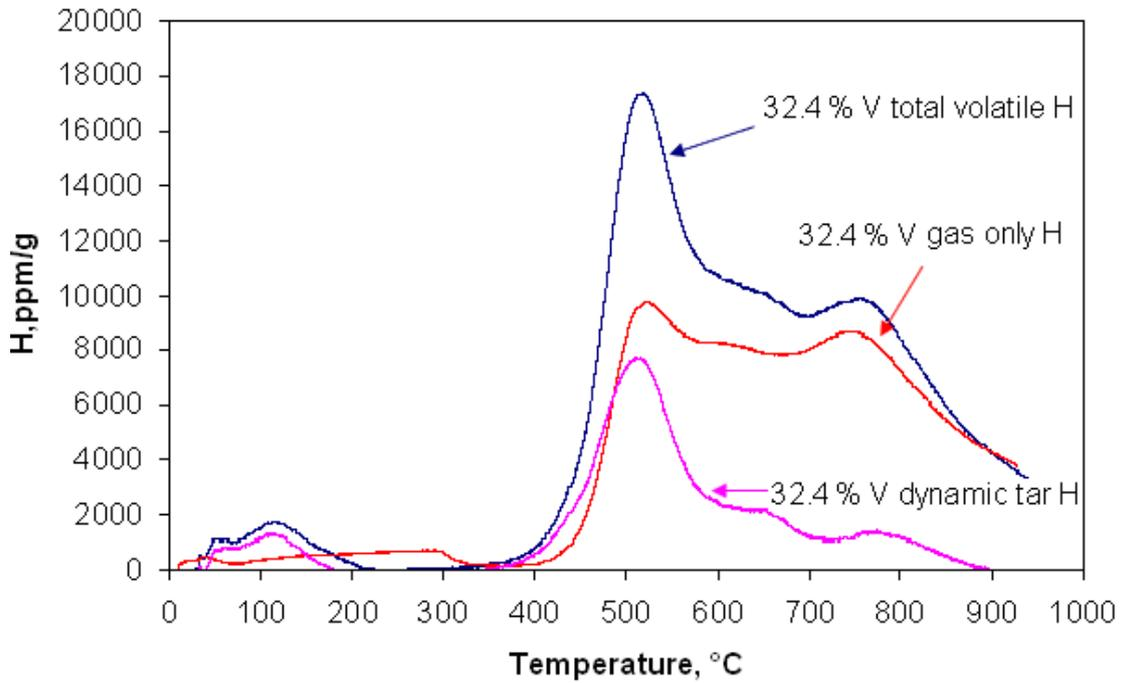
**Figure 8.9. Hydrogen concentration for total volatile, gas only and mathematically derived dynamic tar for the 32.4% vitrinite concentrate at a heating rate of 10°C/min from 25 to 1000°C.**
