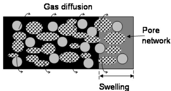
(d) Gas flow is restricted to diffusion through the liquid metaplast and a pore network forms (450-510°C), the swelling portion is indicated by a different colour to the original coal bed.
