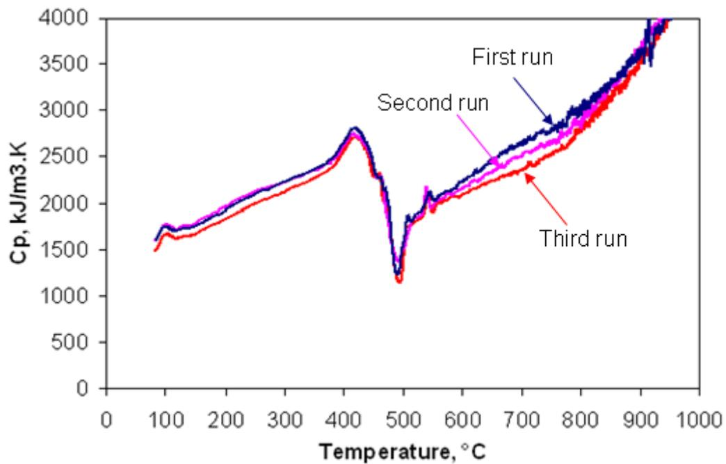
Figure 7.4. Apparent specific heat of the 86.4% vitrinite concentrate at a heating rate of 10°C/min from 25 to 1000°C for three replicate experiments.
