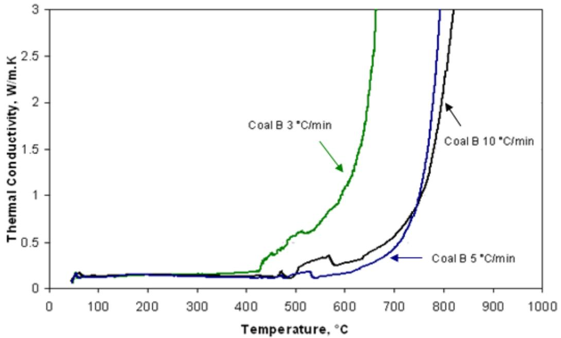
Figure 4.17. Thermal conductivities of coal sample B at three different heating rates of 3, 5 and 10°C/min from 25 to 1000°C.
