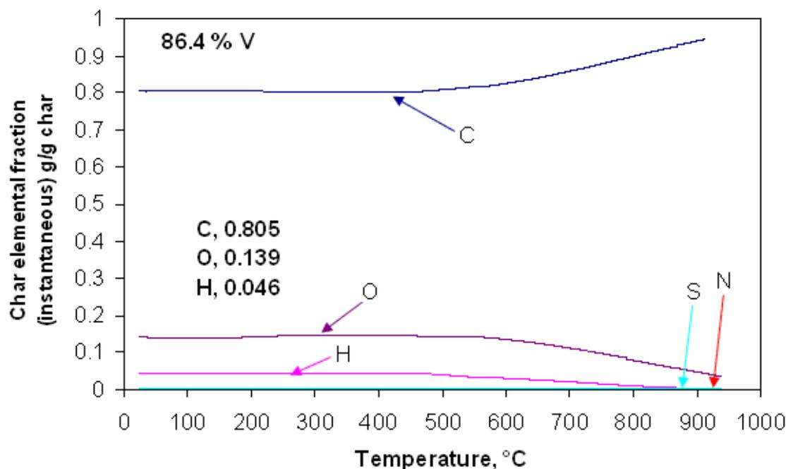
Figure 8.16. Calculated elemental compositions of the residue as a function of temperature for the 86.4% vitrinite concentrate at a heating rate of 10°C/min from 25 to 1000°C.
