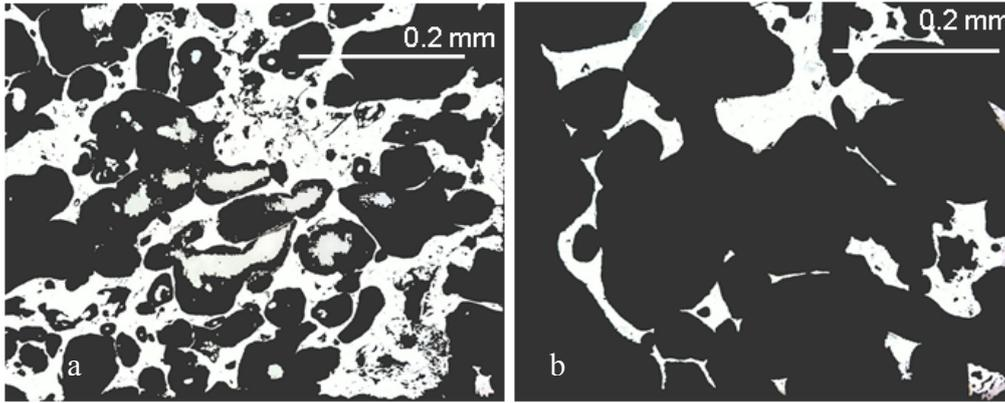
**Figure 4.12. Optical microscopy images of cokes obtained from 0-212  $\mu\text{m}$  coal sample B at the heating rate of  $3^\circ\text{C}/\text{min}$  (a) and  $10^\circ\text{C}/\text{min}$  (b), both images obtained near the centre of the cross section of the cylinder coke sample.**
