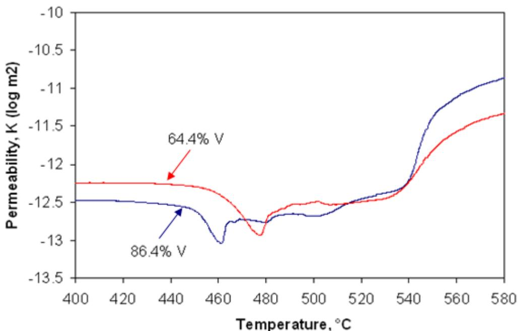
Figure 7.11. Estimated permeability based on Darcy law for coal maceral concentrates at a heating rate of 10°C/min.
