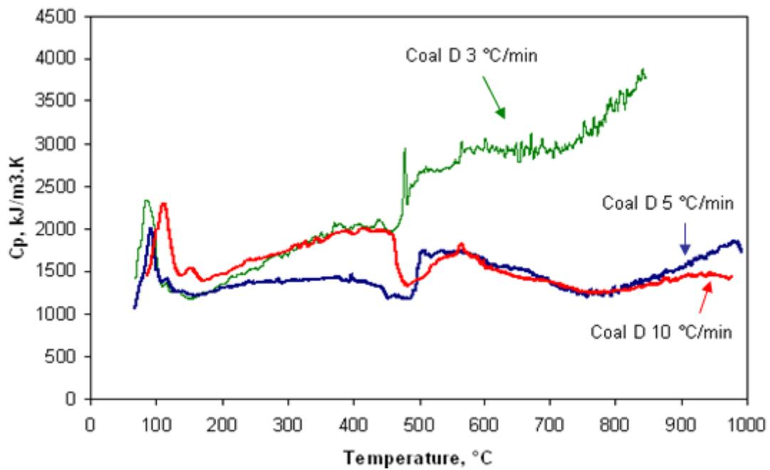
Figure 4.15. Apparent specific heat of coal sample D at three different heating rates of 3, 5 and 10°C/min from 25 to 1000°C.
