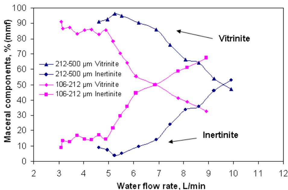
**Figure 6.1. Coal maceral components versus water flow rate within the reflux classifier for all 106-212  $\mu\text{m}$  and 212-500  $\mu\text{m}$  size cuts of coal maceral concentrates.**
