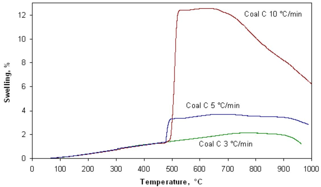
Figure 4.9. Swelling of coal sample C at three different heating rates of 3, 5 and 10°C/min from 25 to 1000°C.
