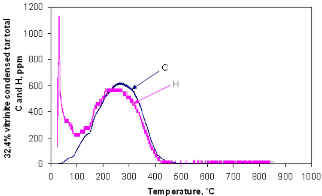
Figure 8.24. Properties of condensed tar obtained from the 32.4% vitrinite concentrate at a heating rate of 10°C/min from 25 to 505°C.
