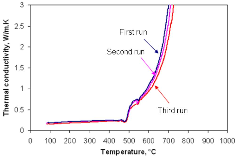
**Figure 7.5. Thermal conductivity of the 86.4% vitrinite concentrate at a heating rate of 10°C/min from 25 to 1000°C for three repeated experiments.**
