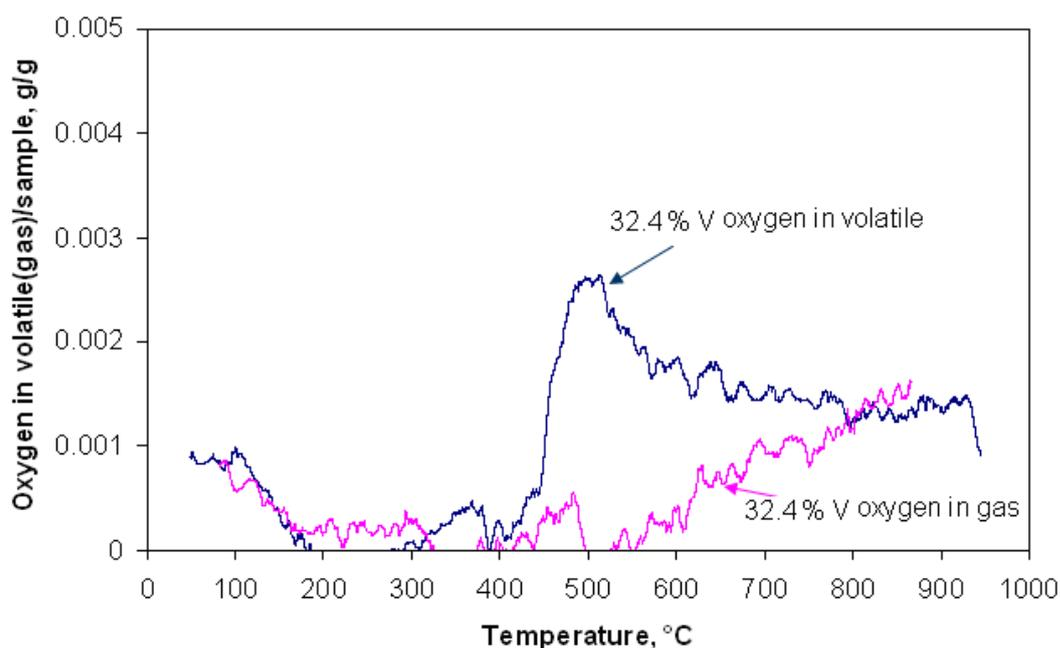
**Figure 8.15. Oxygen in volatile matter and gas only for the 32.4% vitrinite concentrate at a heating rate of 10°C/min from 25 to 1000°C.**
