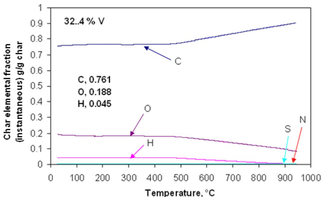
Figure 8.17. Calculated elemental compositions of the residue as a function of temperature for the 32.4% vitrinite concentrate at a heating rate of 10°C/min from 25 to 1000°C.
