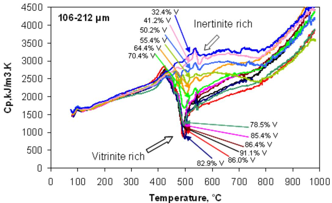
Figure 6.7. Apparent specific heat for 106-212  $\mu\text{m}$  coal maceral concentrates at a heating rate of  $10^\circ\text{C}/\text{min}$  from 25 to  $1000^\circ\text{C}$ .
