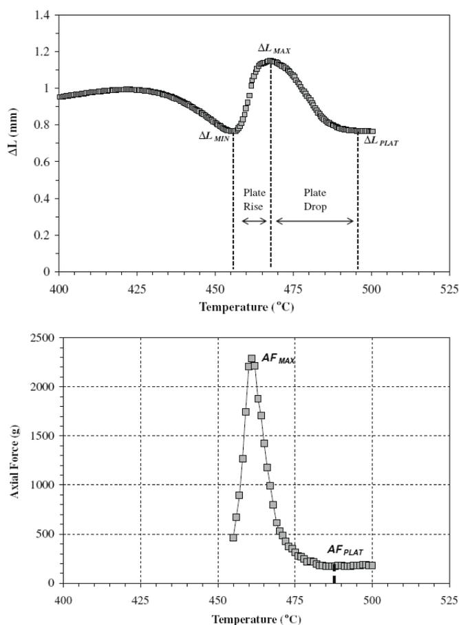
Figure 2.8. (Top) Plate displacement  $\Delta L$  as a function of temperature for one coking coal (71% vitrinite), (bottom) axial force (AF) as a function of the same coal [88].
