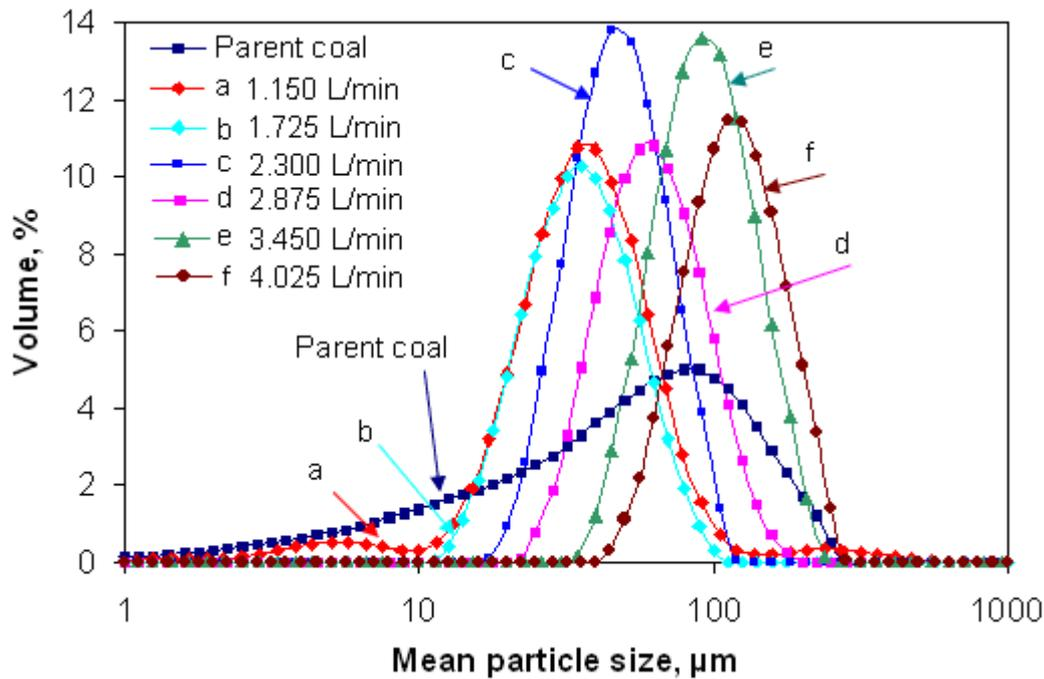
Figure 5.1. Mean particle size analysis of the parent coal C and separated coal maceral concentrates.
