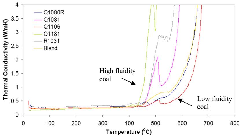
**Figure 2.16. Effective thermal conductivity for the coal samples at a heating rate of 5°C/min heated from room temperature to 1000°C [19].**
