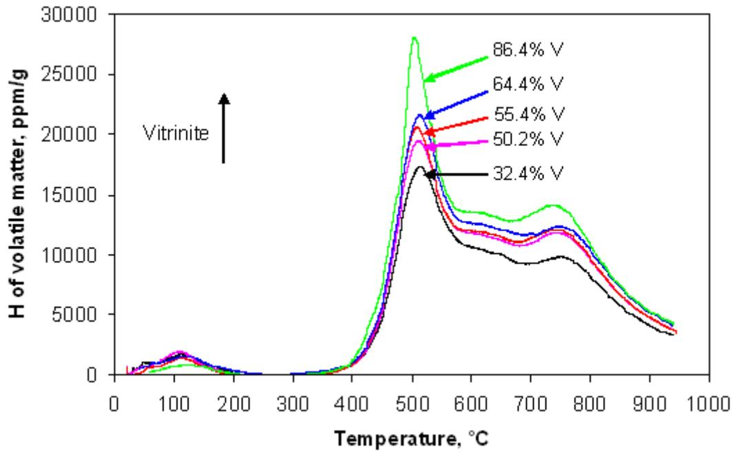
Figure 8.2. Hydrogen concentration of total volatiles for various coal maceral concentrates at a heating rate of 10°C/min from 25 to 1000°C.
