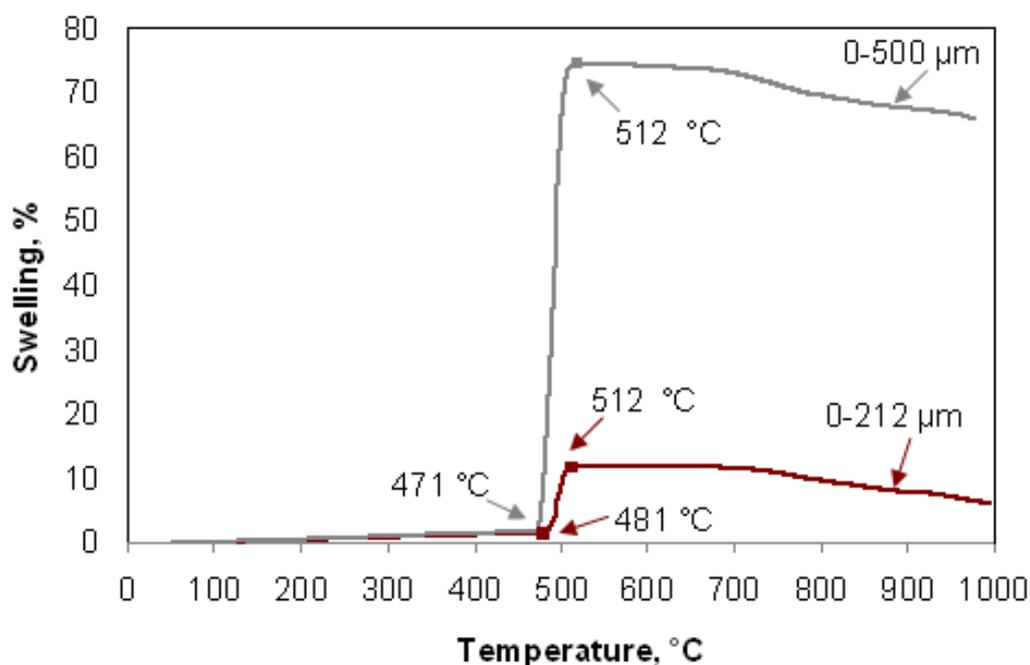
**Figure 4.21. Effect of particles size on swelling for coal sample C at a heating rate of 10°C/min from 25 to 1000°C.**
