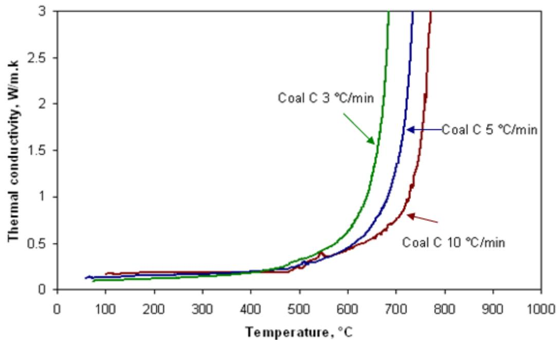
Figure 4.18. Thermal conductivities of coal sample C at three different heating rates of 3, 5 and 10°C/min from 25 to 1000°C.
