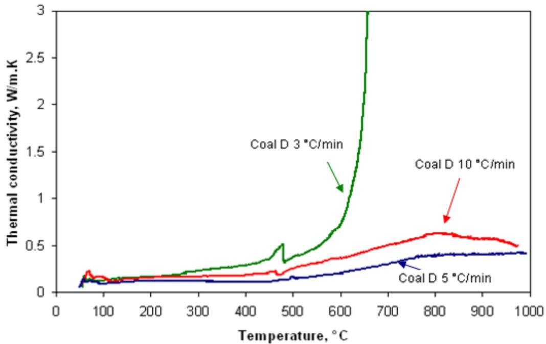
Figure 4.19. Thermal conductivities of coal sample D at three different heating rates of 3, 5 and 10°C/min from 25 to 1000°C.
