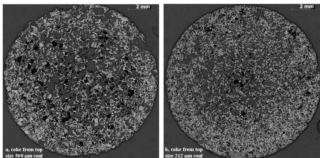
**Figure 4.22. Overview of optical microscopy images of cokes formed from coal sample C at a heating rate of 10°C/min from 25 to 1000°C; (a) coke formed from 0-500 μm particle size coal, (b) coke formed from 0-212 μm particle size coal.**
