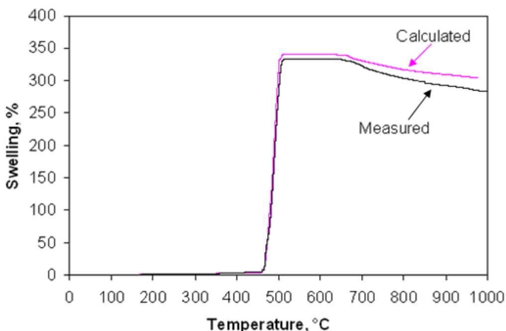
Figure 6.11. Calculated by mass average and measured swelling for a blend of 85.4% vitrinite concentrate with a particle size of 106-212  $\mu\text{m}$  and 85.7% vitrinite concentrate with a particle size of 212-500  $\mu\text{m}$ , blended at a ratio of 1:1 by mass, at a heating rate of 10°C/min from 25 to 1000°C.
