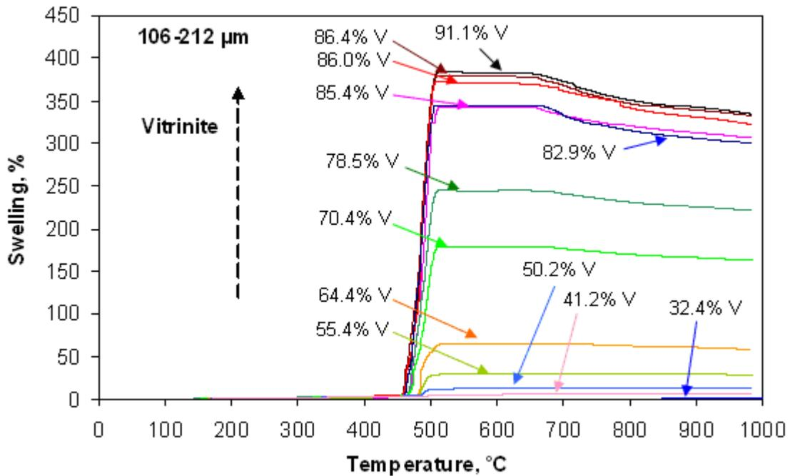
Figure 6.5. Swelling for 106-212  $\mu\text{m}$  coal maceral concentrates at a heating rate of  $10^\circ\text{C}/\text{min}$  from 25 to  $1000^\circ\text{C}$ .
