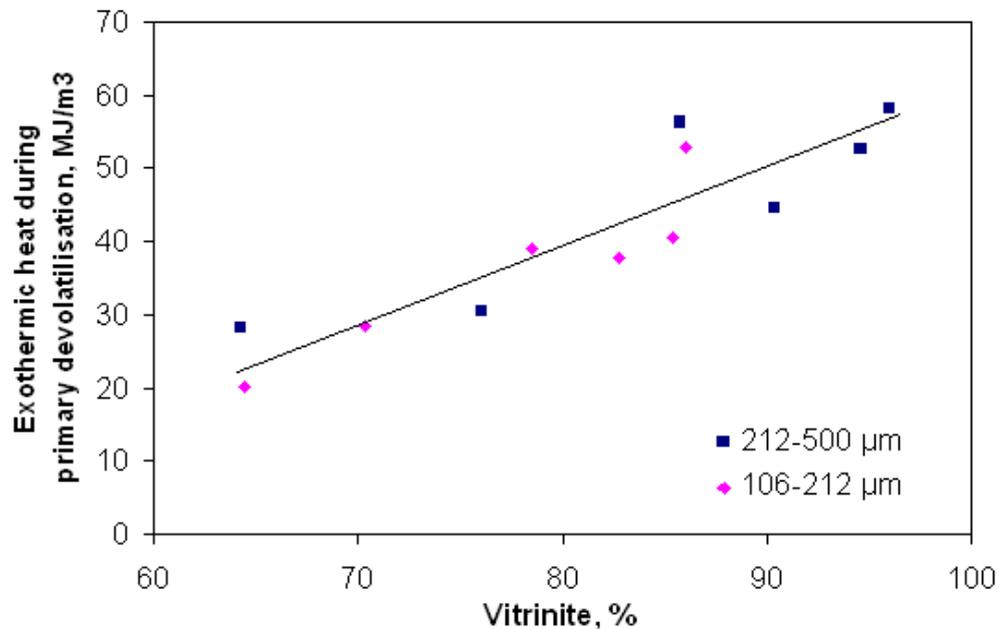
Figure 6.19. Relationship between exothermic heat during the primary devolatilisation (420-540°C) and vitrinite content for the 106-212  $\mu\text{m}$  and 212-500  $\mu\text{m}$  size cuts of coal maceral concentrates at a heating rate of 10°C/min.
