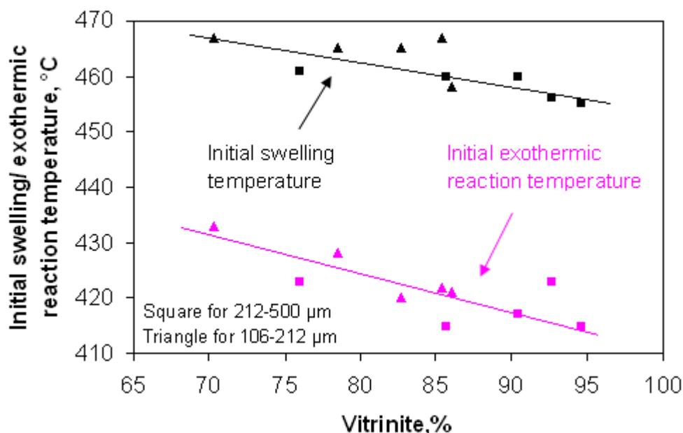
**Figure 6.21. Relationship between the temperatures for the onset of swelling, primary exothermic reaction and the vitrinite content for the 106-212  $\mu\text{m}$  and 212-500  $\mu\text{m}$  size cuts of coal maceral concentrates at a heating rate of  $10^\circ\text{C}/\text{min}$ .**
