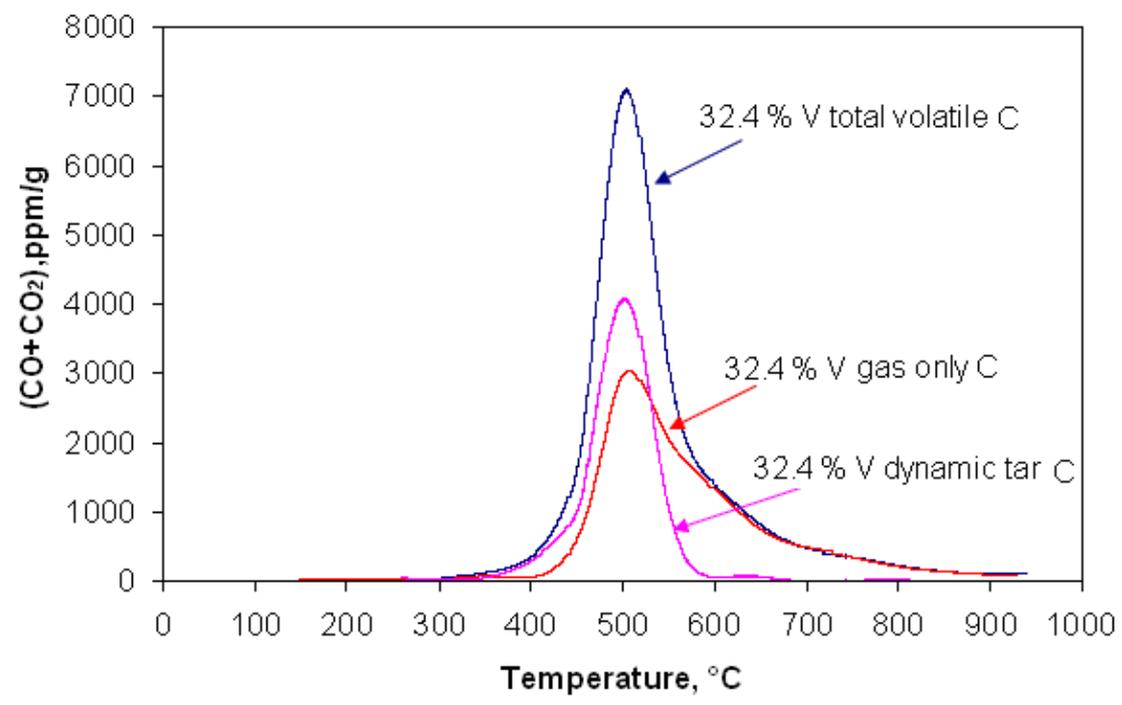
**Figure 8.10. Carbon concentration for total volatile, gas only and mathematically derived dynamic tar for the 32.4% vitrinite concentrate at a heating rate of 10°C/min from 25 to 1000°C.**
