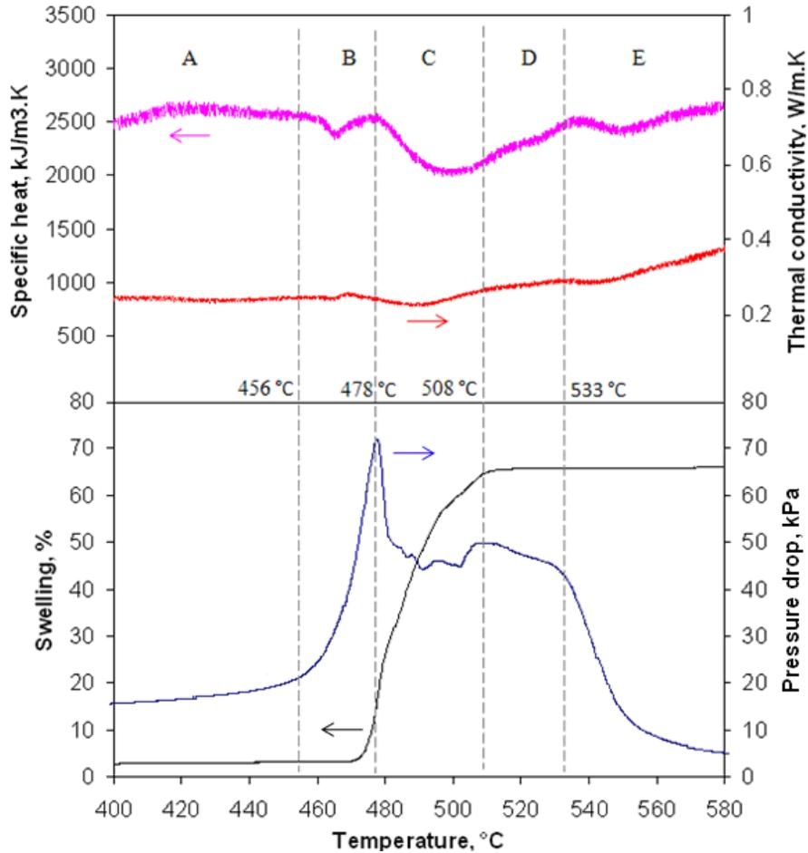
**Figure 7.7. Correlation between swelling, pressure drop of gas flowing through the coal sample, apparent specific heat and thermal conductivity for the 64.4% vitrinite concentrate at a heating rate of 10°C/min.**
