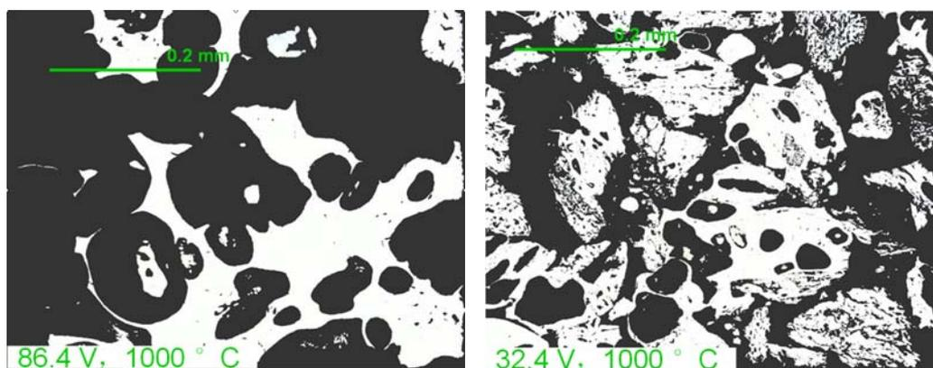
Figure 6.17. Optical microscopy images of coke obtained from 106-212  $\mu\text{m}$  (a) 86.4% vitrinite concentrate, (b) 32.4% vitrinite concentrate at a heating rate of 10°C/min from 25 to 1000°C, both images obtained near the centre of the cross section of the cylinder coke sample.
