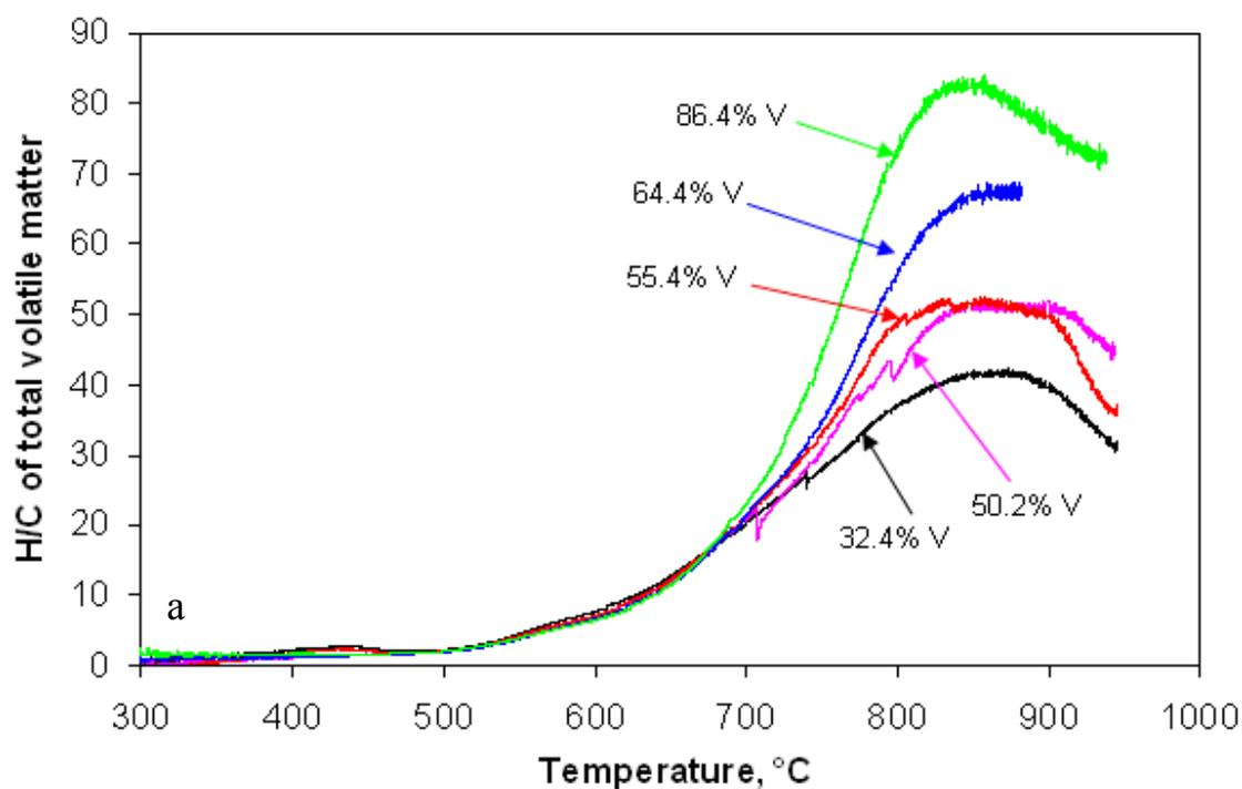
Figure 8.4 (a). The H/C of total volatiles for various coal maceral concentrates at a heating rate of 10°C/min from 25 to 1000°C.
