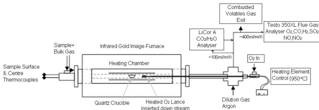
**Figure 3.4. DETA apparatus for measurements of chemical compositions (CHNOS) of tars and gases during evolution.**
