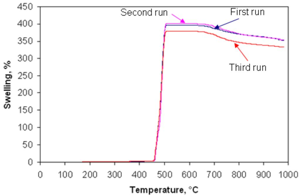
Figure 7.1. Swelling of the 86.4% vitrinite concentrate at a heating rate of 10°C/min from 25 to 1000°C for three replicate experiments.
