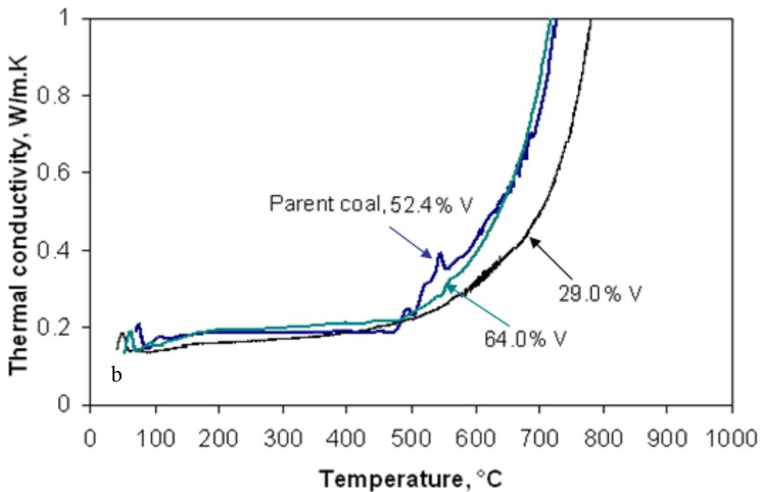
Figure 5.4 (b). Thermal conductivity of the parent coal C and two inertinite rich concentrates separated from the parent coal C at a heating rate of 10°C/min from 25 to 1000°C.
