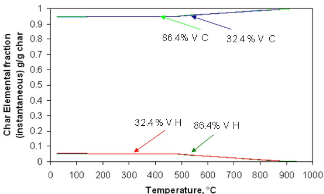
Figure 8.19. Calculated elemental compositions of the residue as a function of temperature for the 86.4% and 32.4% vitrinite concentrates at a heating rate of 10°C/min from 25 to 1000°C (with carbon and hydrogen only considered).
