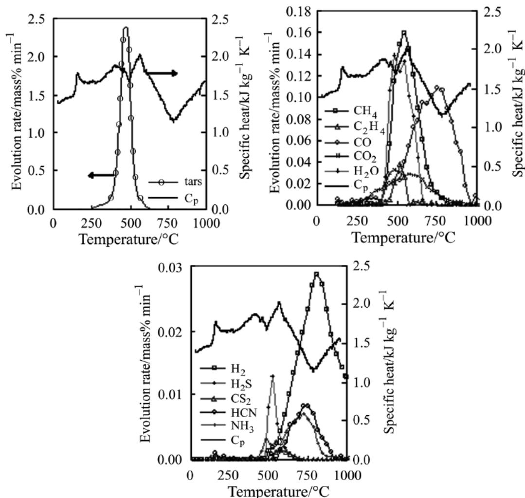
Figure 2.10. Evolution rate of tars and volatiles of heating coal at a heating rate of 10°C/min [63].
