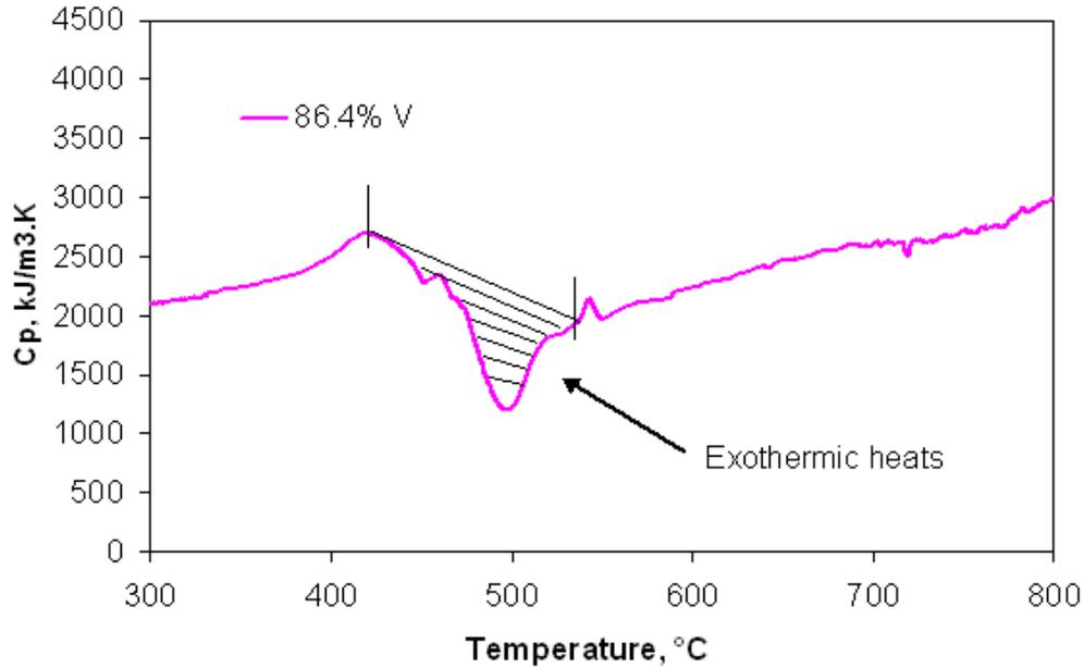
Figure 6.18. A typical example for the calculation of heat of the exothermic reaction during the primary devolatilisation (420-540°C) for the 86.4% vitrinite concentrate with 106-212  $\mu\text{m}$  size range at a heating rate of 10°C/min.
