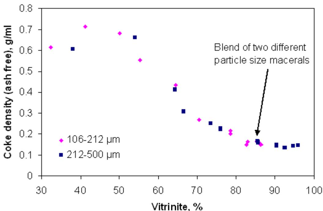
**Figure 6.23.** Coke densities (ash free) against vitrinite content for all coal maceral concentrates at a heating rate of 10°C/min from 25 to 1000°C.
